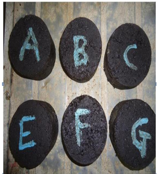
Source: Assefa Feysa Hot Mix Asphalt Concrete Specimen
