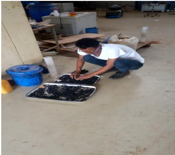
Source: Tesfaye Meshesha Uncompact hot mix asphalt specimen
