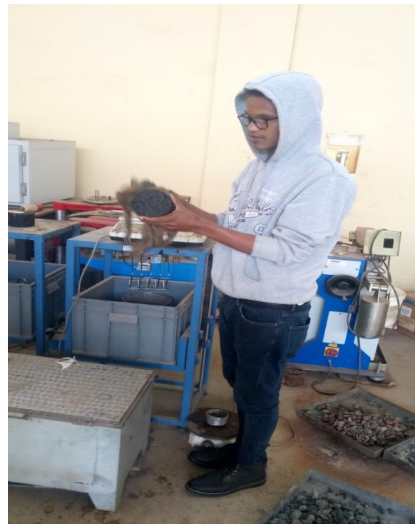
Source: Assefa Feysa Making dry by cloth after weight in water.
