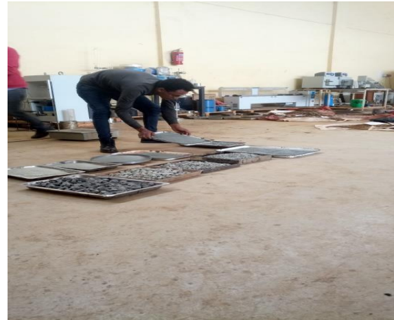
Source: Assefa Feysa Arrange the aggregates by each size.
