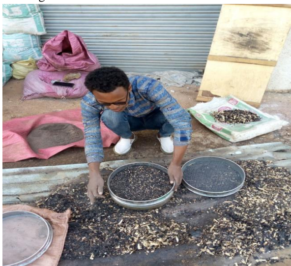
Source: Terefe Marito Burnt Saw dust and sieve to prepare ash.
