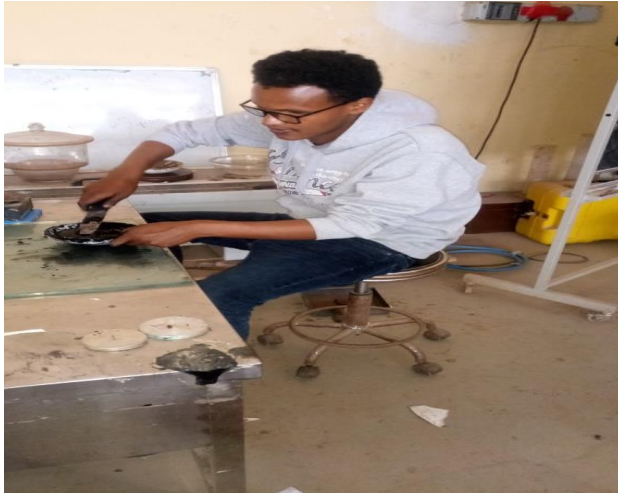
Source: Assefa Feysa Soaking the CCA and SDA
