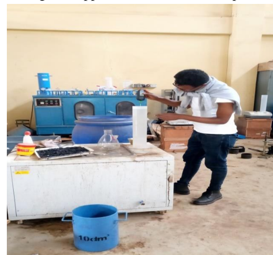
Source : Assefa Feysa Measuring the water Temperature.
