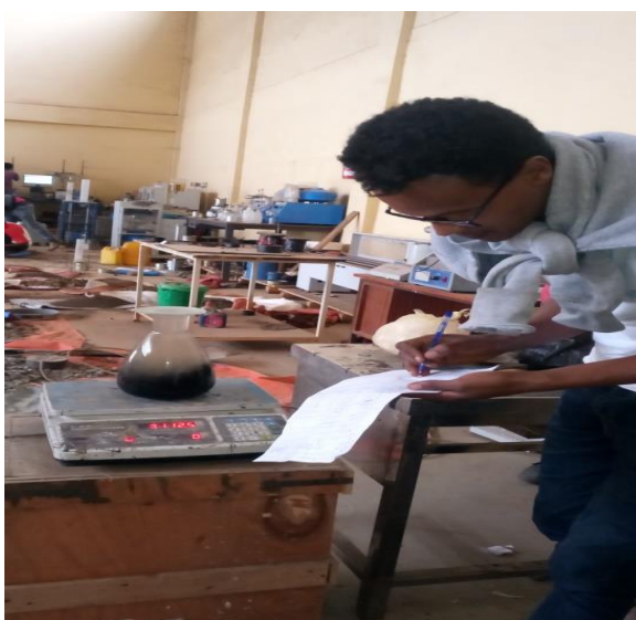
Source: Terefe Marito Recording the weight for Gmm
