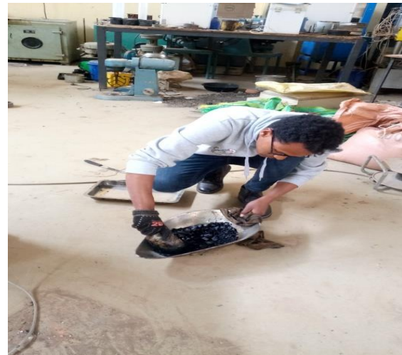
Source: Dejene Dereje Mixing before compactio
