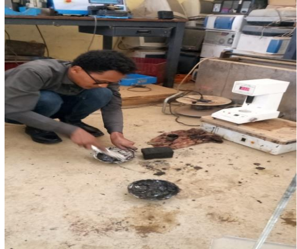
Source: Assefa Feysa Ready the sample for liquid limit test
