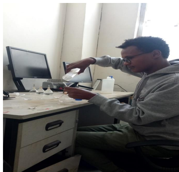
Source: Terefe Marito Fill water in pycnometer jar.
