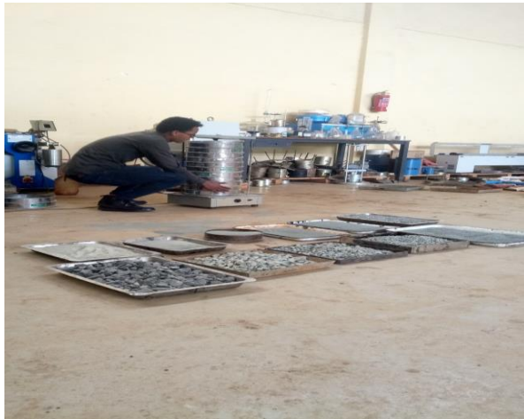
Source: Assefa Feysa Sieve the aggregates by different sieve number.
