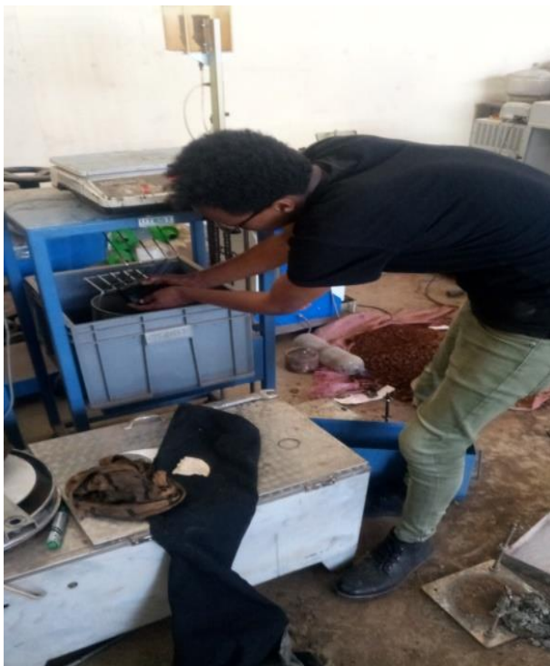
Source: Assefa Feysa Weighting the hot mix asphalt specimen in water.
