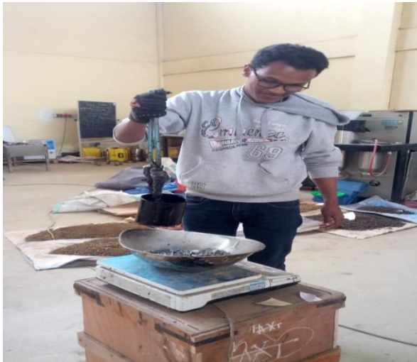
Source: Dejene Dereje Add bitumen on heated aggregates.
