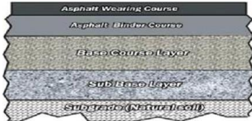
Figure 2. 1: Typical flexible pavement structure layers (Mohammed, 2013)
