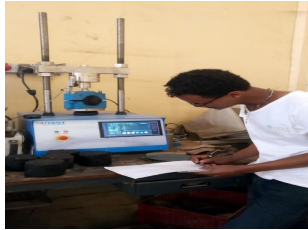
Source: Assefa Feysa recording the Marshall Test results
