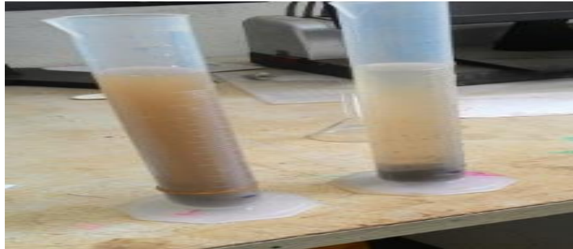
Figure 3. 6 The process of testing free swell (2:00AM, August 29/2019)
