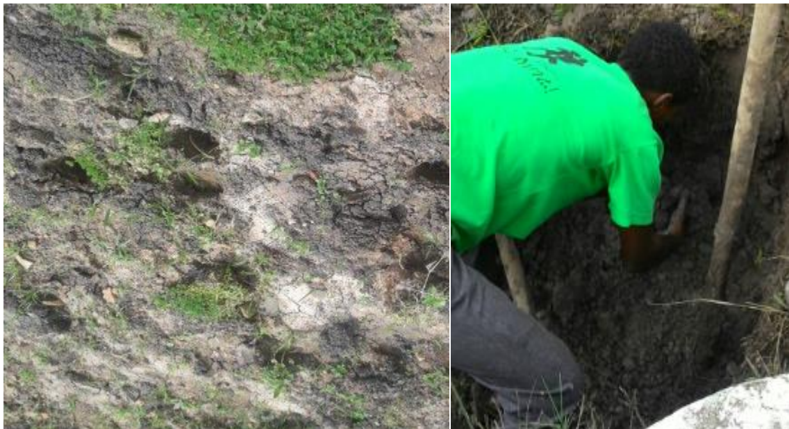
Figure 3. 3 Photo of Expansive Soil Observed and Sampled along Mettu-Burusa road (5:10AM, July22/2019)
