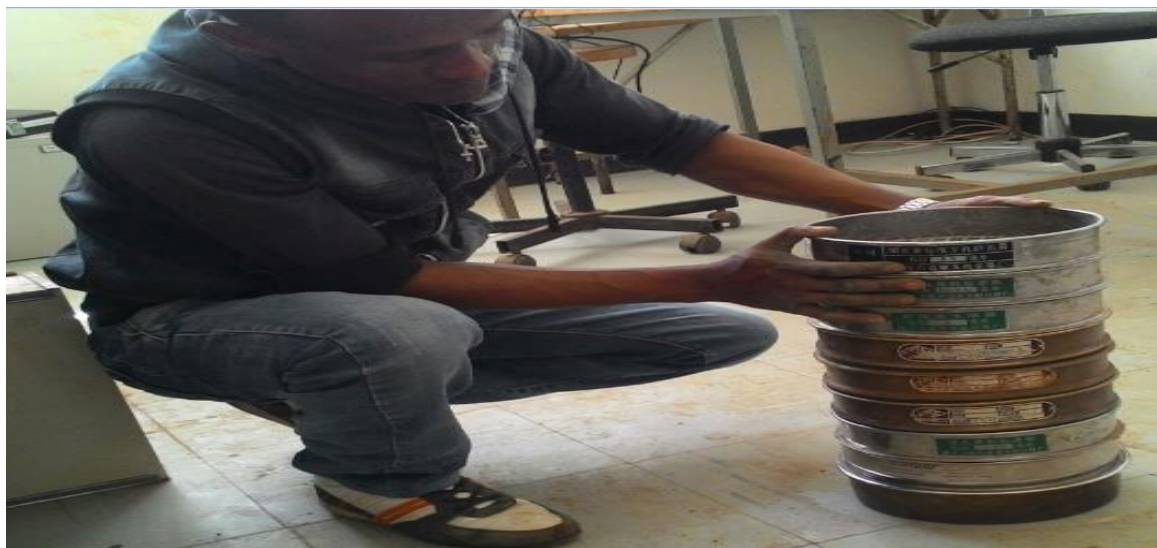
Figure 3. 4 The process of shaking the soil manually (9:25PM, August 21/2019)
