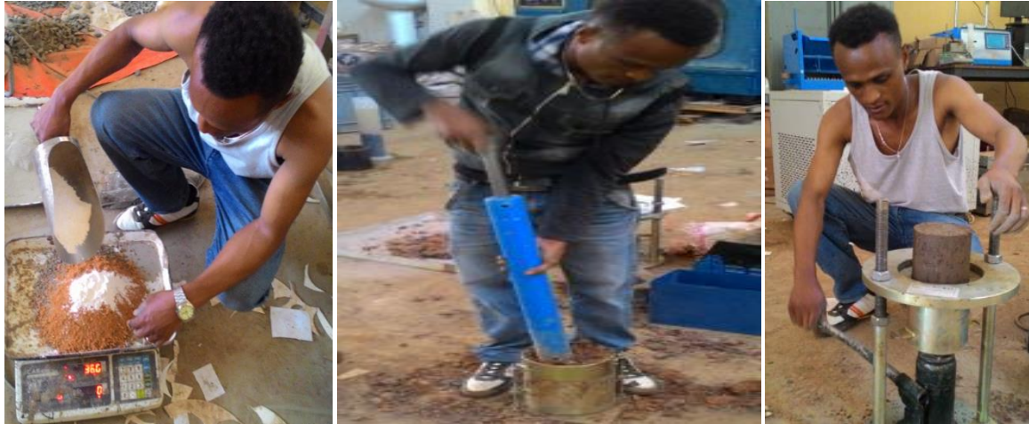
Figure 3. 8 The process of compaction (4:00AM, August 21/2019)
