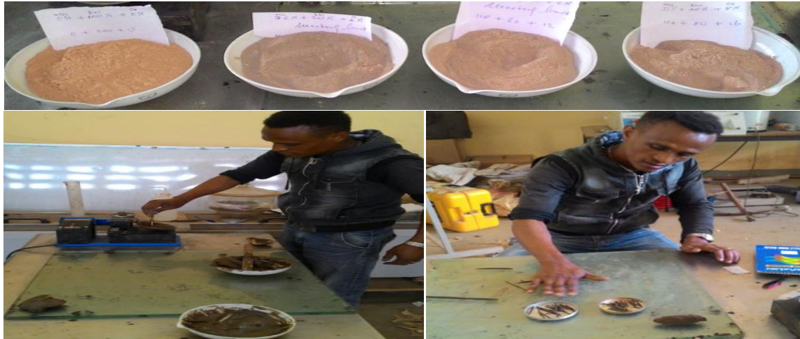
Figure 3. 5 The process of determining Atterberg limit (10:30PM, August 29/2019)
