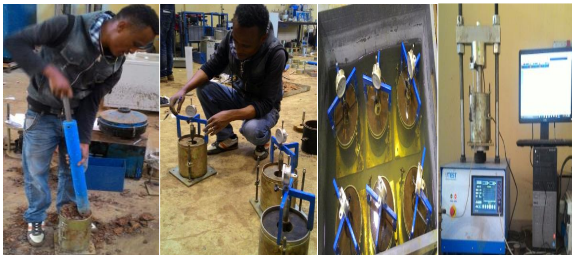
Figure 3. 9 determination of CBR value and CBR-Swell (2:30AM, August 28/2019)
