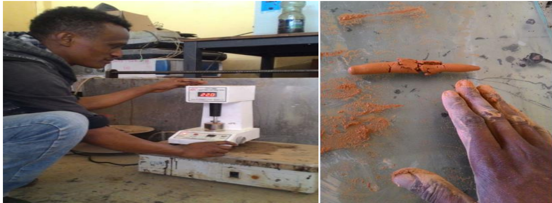
Figure 4. 6 Determination of Atterberg limit of Brick (2:40AM, August 30/2019)
