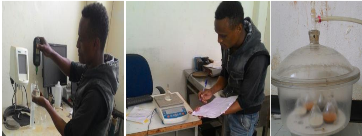
Figure 3. 7 The process of determining specific gravity (11:30PM, August 29/2019)
