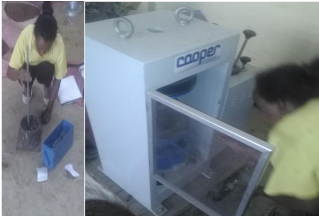
Figure 3.11: Crushing Value Test and apparatus to crush aggregate [Terefe 27, 3:45]
