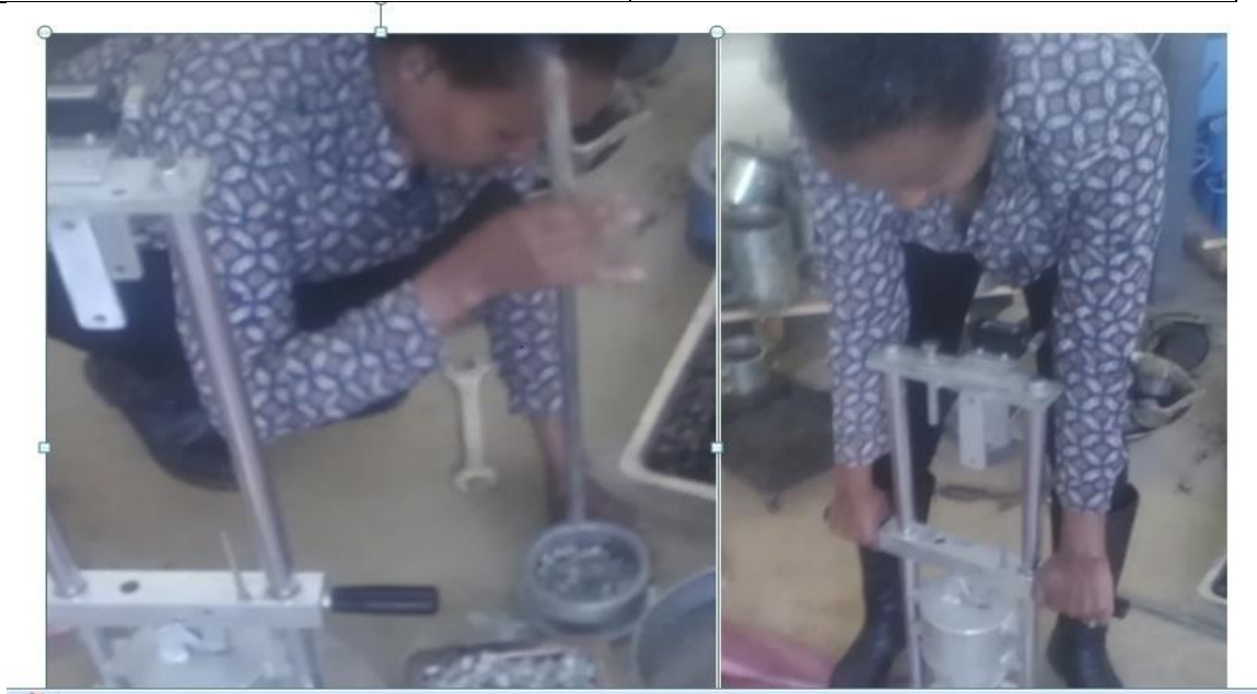
Figure 3.12: Aggregate impact value test and apparatus used [Tigist25, 4:08]
