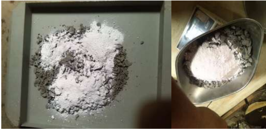
Figure 2: Blending of Crushed stone sub-base material with AMASSA byproduct (Date: 28/05/2016)
