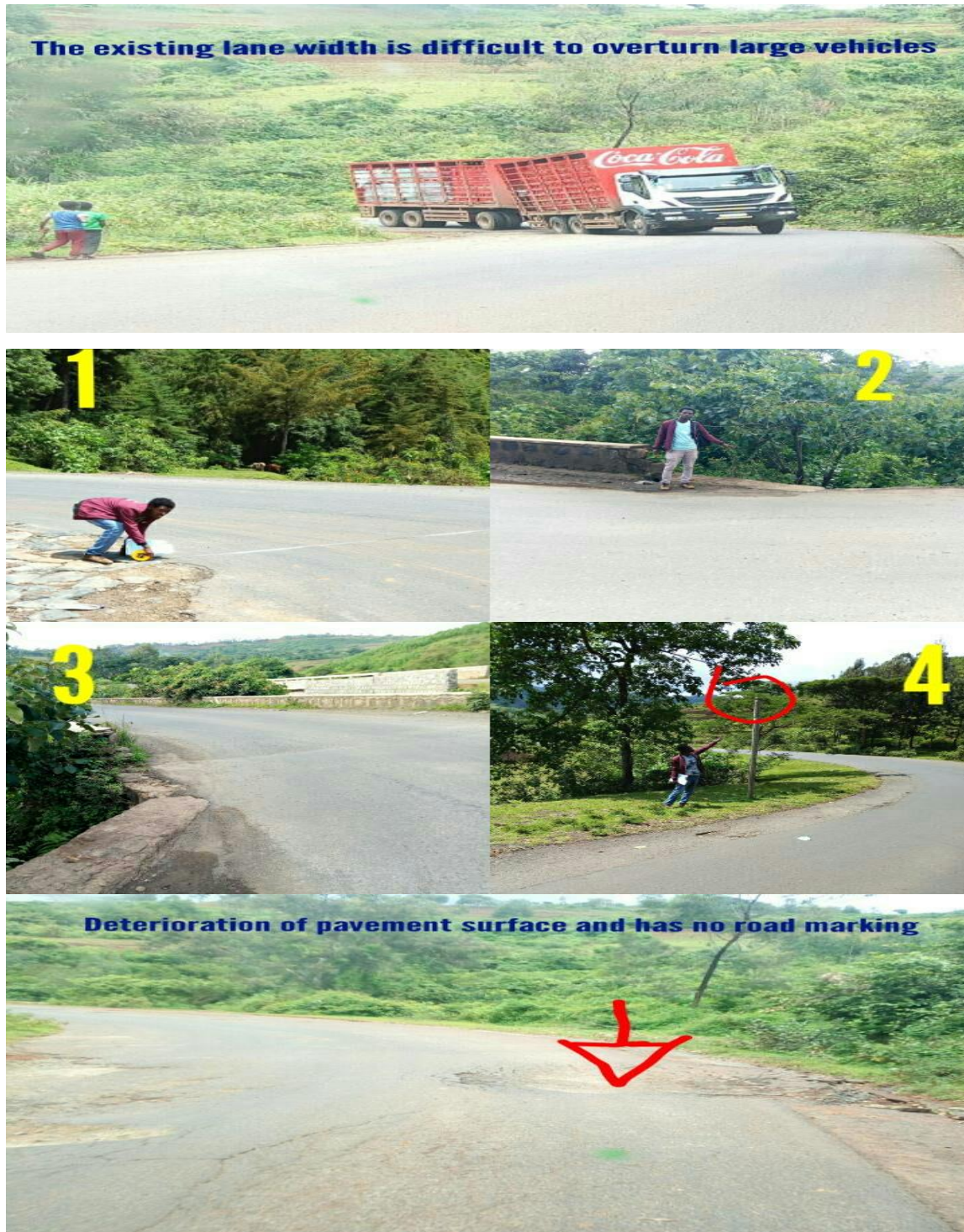
Photo No. 1: road safety audit such as measurements lane width, shoulders width
