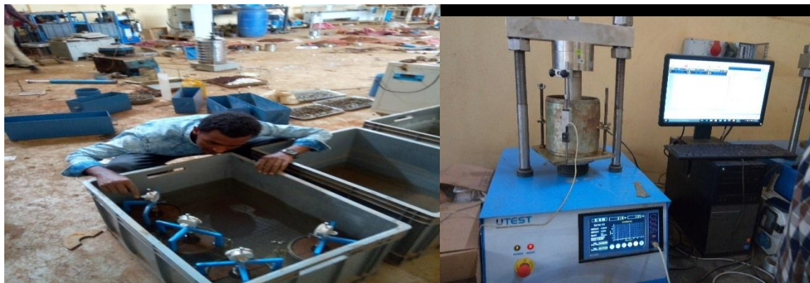
Figure 3-5: CBR determinations (August 9, 2011, 3:15 by Diriba)
