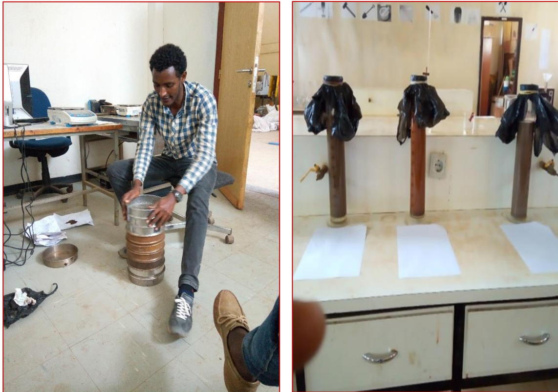
Figure 3-9: Sieve and hydrometer analysis (August 20, 2011, 8:15 PM by Aseffa)
