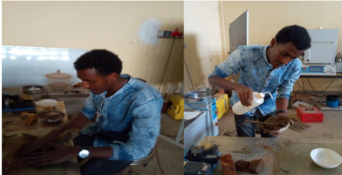
Figure 3-6: Atterberg's determination for the soil (August 10, 2011, 3:15 AM by Aseffa)
