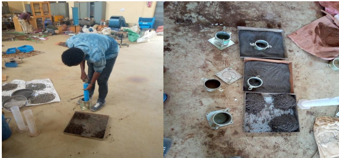
Figure 3-4: Determinations of MDD and OMC (August 1, 2011, 3:15 AM by Diriba)
