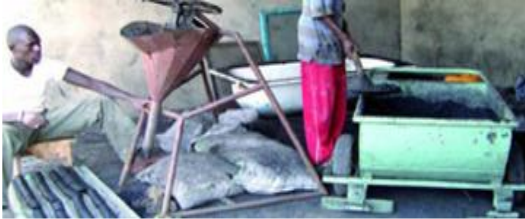
Figure 2.4 Briquetting charcoal dust in Saint-Louis using the rotor press (Nederland's Ministry of Economic Agency, 2013)
