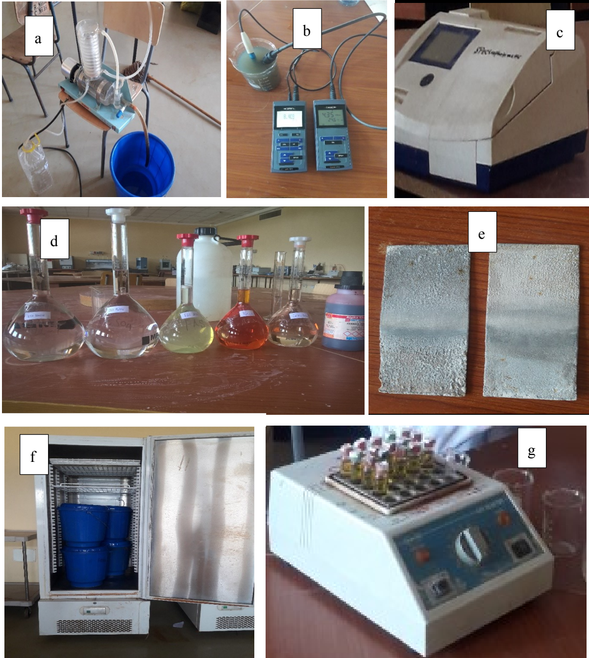
Figure 3-5 a) Distiller b) pH and conductivity meter c) spectrophotometer d) Reagents e) Al electrodes f) Laboratory refrigerator g) COD reactor used in Laboratory
