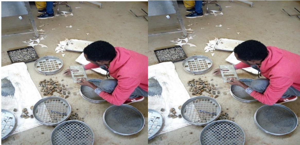
Figure 3.8: photo taken during flakiness index test (Source: Nasir Faris)
