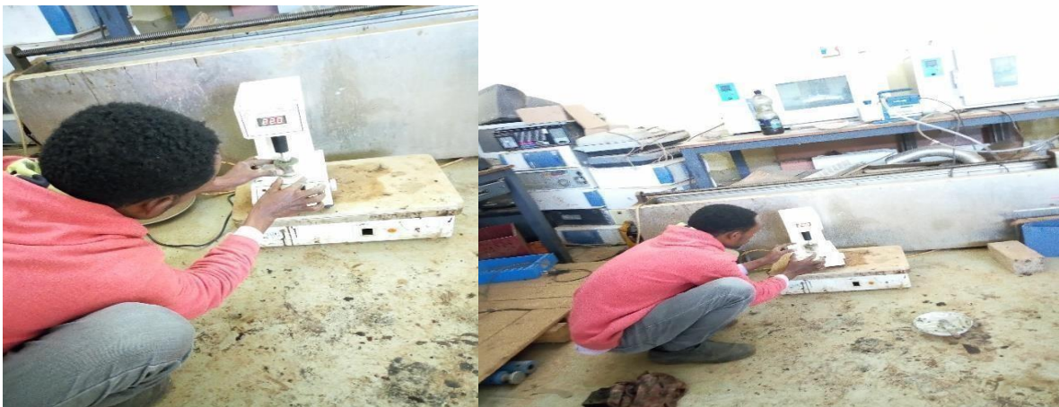
3.5: photo taken during liquid limit test (source: Ahadu Mengiste)
