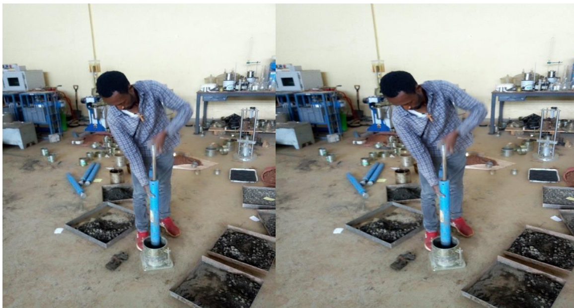
Figure 3.6: photo taken during compaction test for both samples (source: shimelies Agito)
