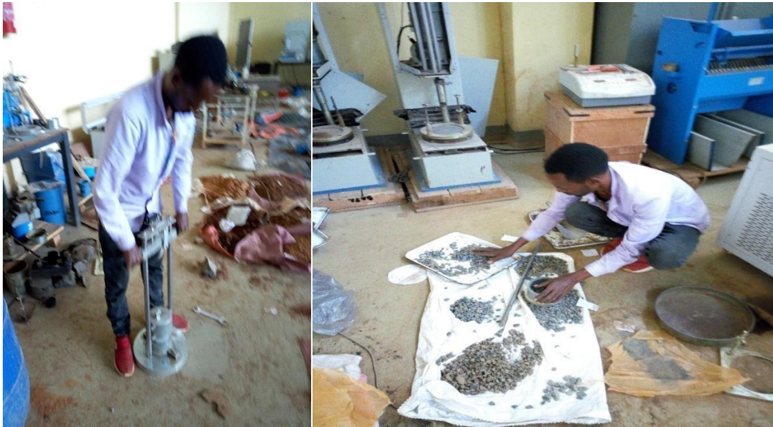
Figure 3.9: photo taken during impact value test (Source: Dejene.D)
