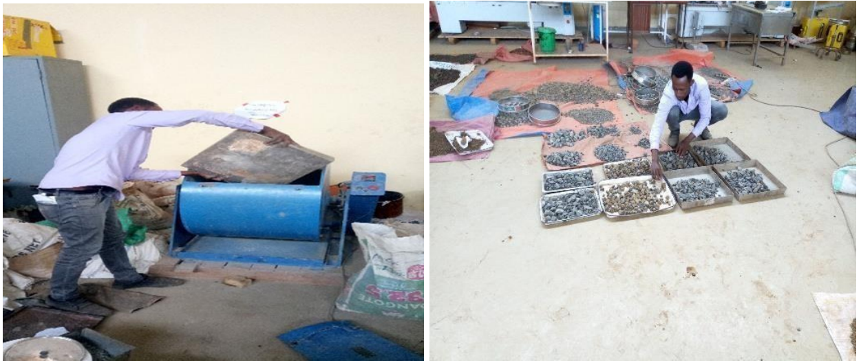
Figure 3.7: photo taken during abrasion test of sample(source: Tesfahun Meshesha)
