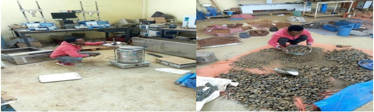
Figure 3.4: photo taken during gradation test for both RG and CSA (source: Merid mesfin)
