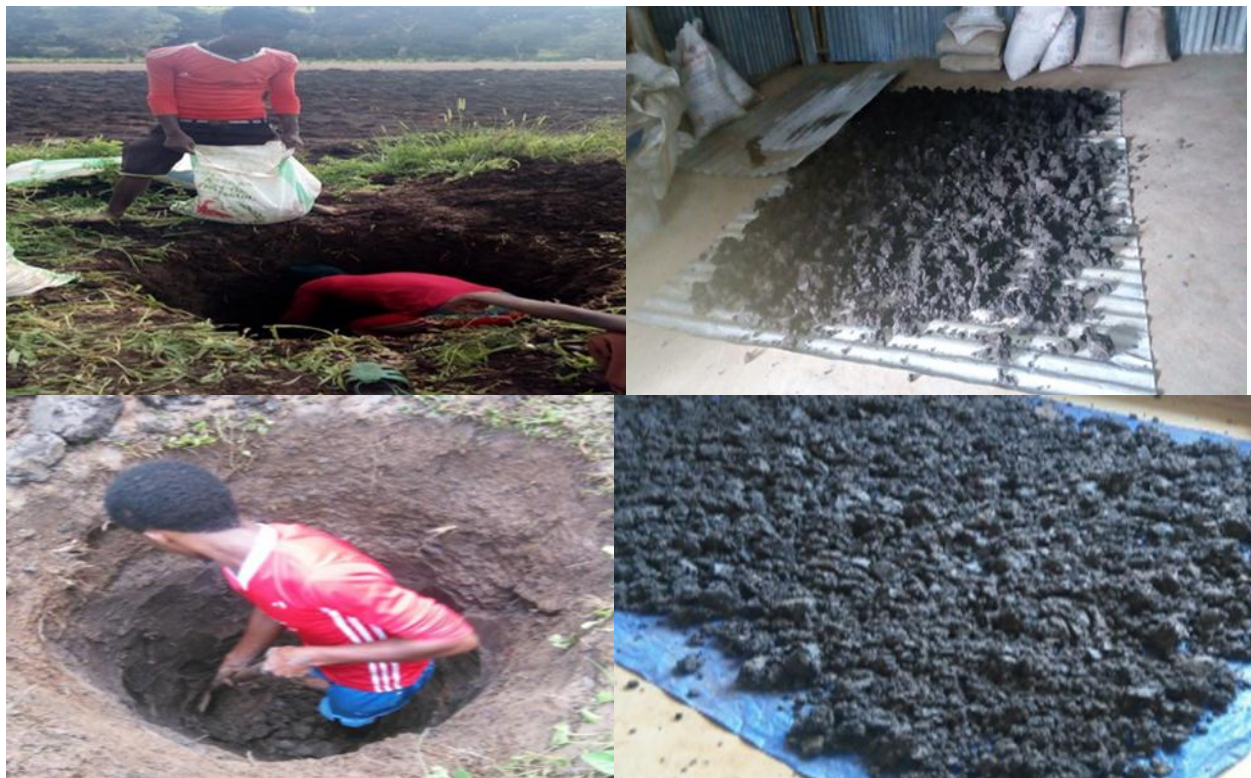
Figure 3. 3:Photo of black cotton soil taken from AABRP and HAP site (source: Gidey T.,2018).
