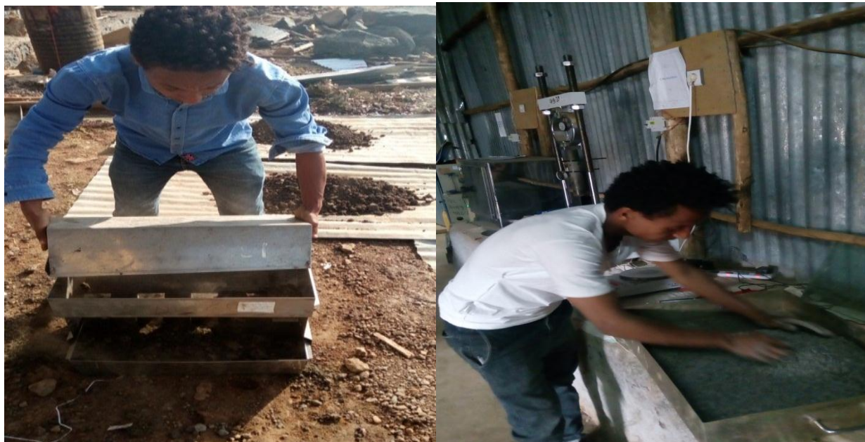
Figure 3. 5: sample quartering and mixing of black cotton soil with bagasse ash and cement (source: Gidey T., 17/112018).
