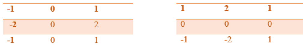
Figure 2.2: The Sobel convolution masks [40]
