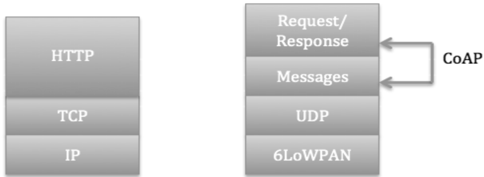
Figure 2. 4: HTTP and CoAP protocol stacks
