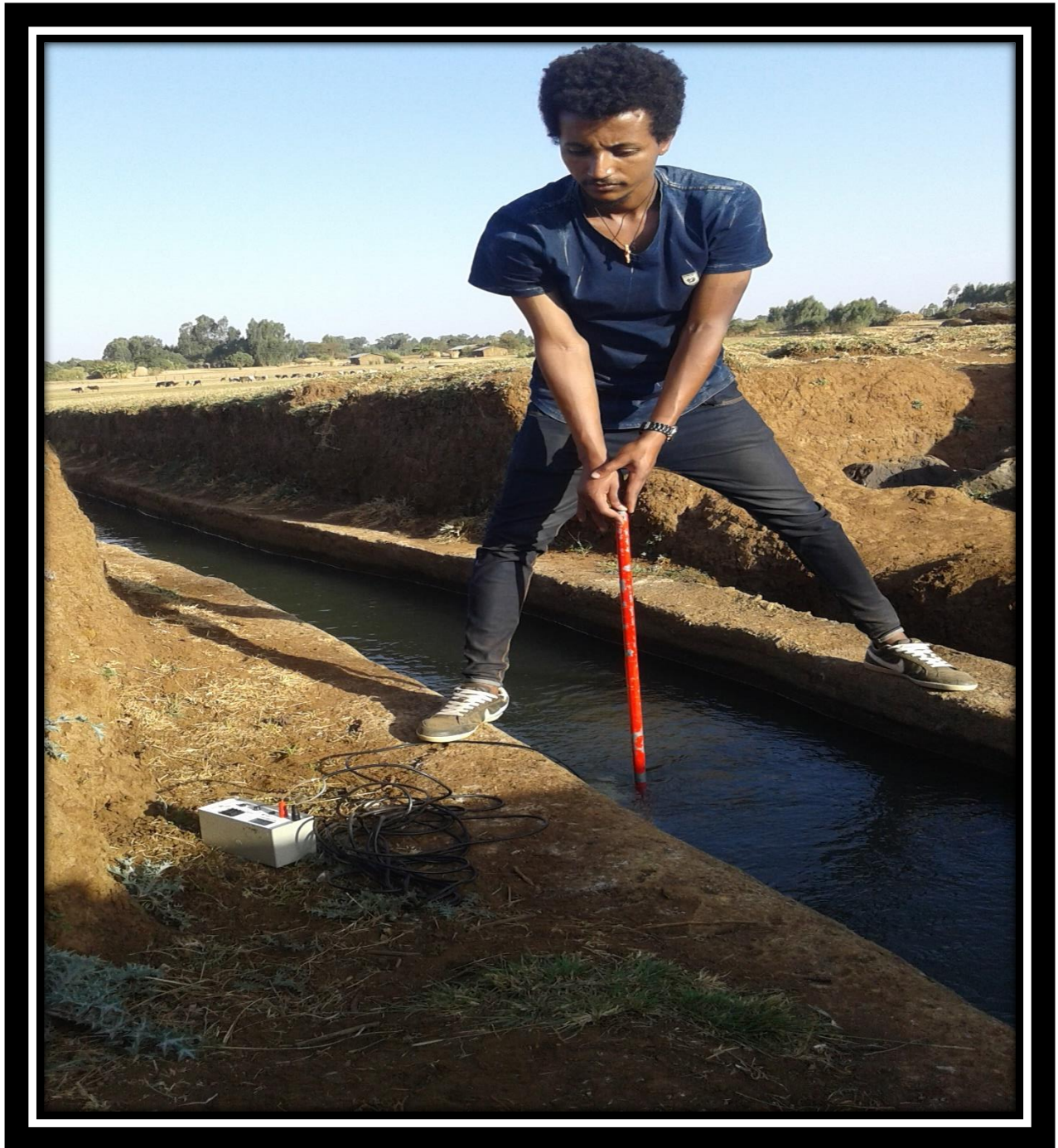
Figure 4.2 measuring conveyance efficiency on main canal of Asher irrigation scheme using current meter
