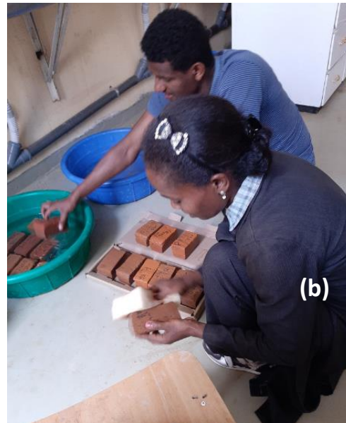
Figure D-2 Researcher (a) marking the samples (b) Taking the sample from water absorption test
