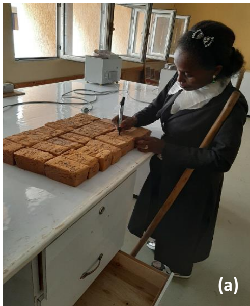
Figure D-2 Researcher (a) marking the samples (b) Taking the sample from water absorption test
