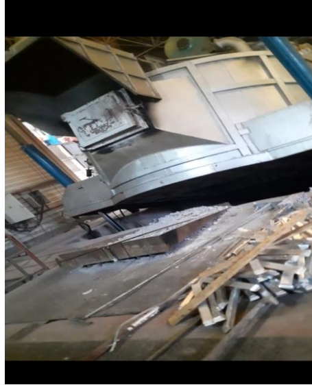
Figure3.4 Shows melt holding furnace
