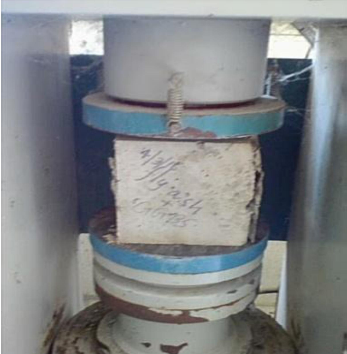
Figure 2.6 Compressive strength test cubic specimen (kumar & Hanitha, 2016)
