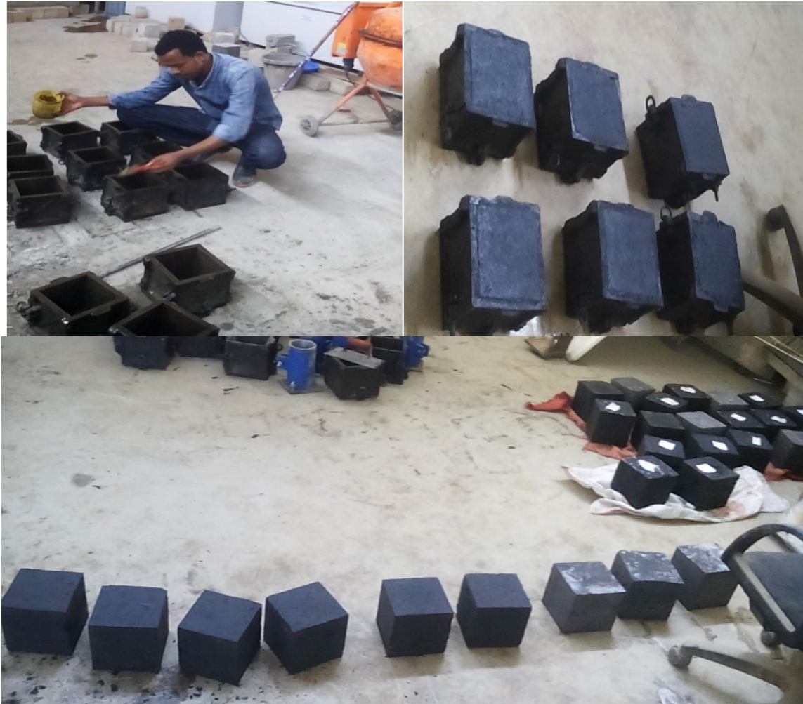
Figure 3.8 Mould preparation, Casting and Curing of Geo-polymer concrete
