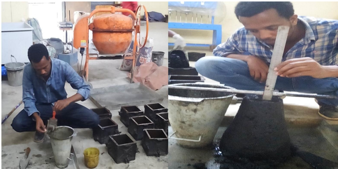
Figure 3.7 Sump Tests of Geo-polymer Concrete
