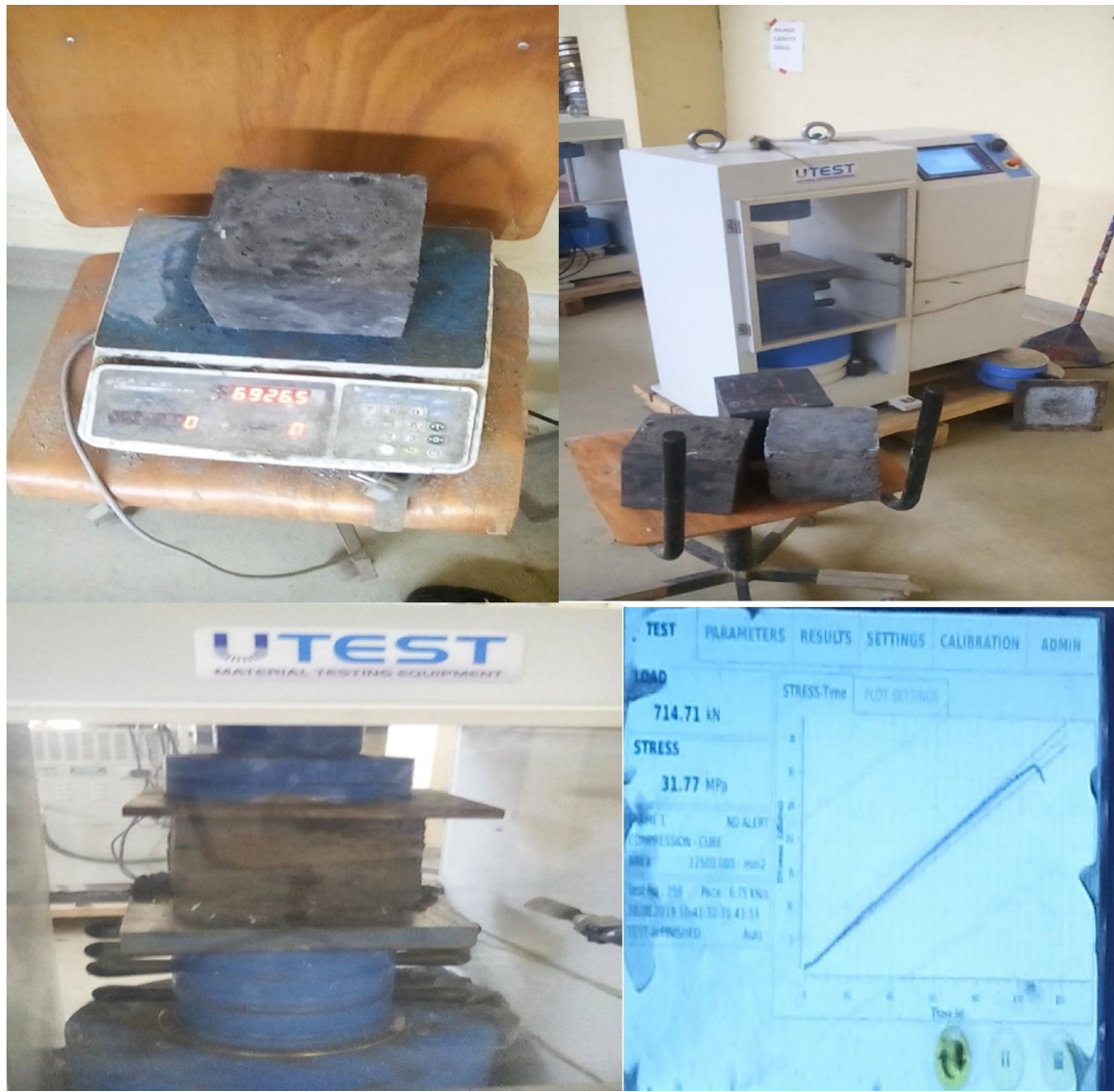
Figure 3.9 Cube Weighting, Compressive Strength Test and Reading
