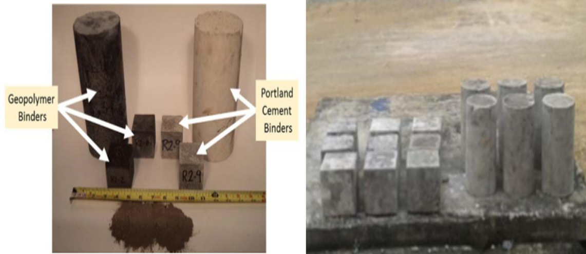
Figure 2.4 Geopolymer concrete Vs OPC concrete (Akbari et al., 2015) and Ambient curing of Geopolymer (Vinodhini et al., 2015)
