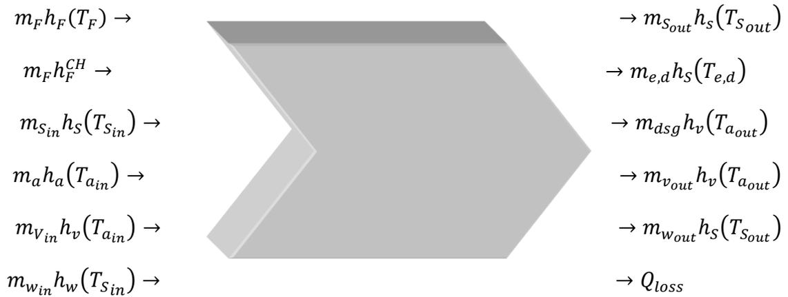
Figure 22: Energy balance in the dryer.
