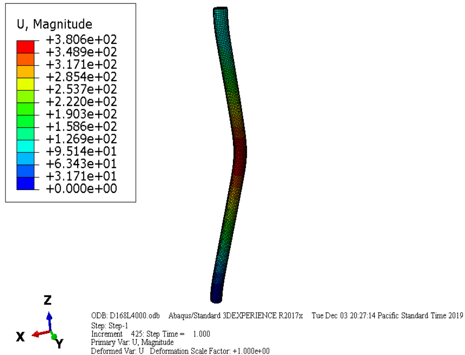
Figure 4.10 Mid-height deflection for M-5
