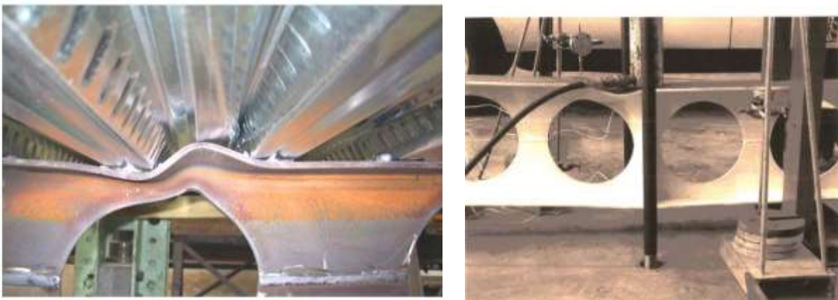
Figure 2. 8: Vierendeel yielding mechanism (Durif, Bouchaïr and Vassart, 2013) and (Warren, 2001)
