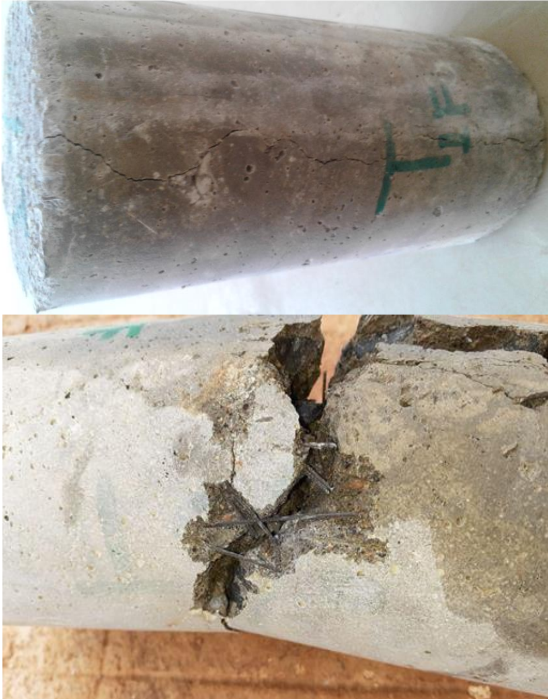
Figure 4. 4: Crushed SFRC cylindrical specimens
