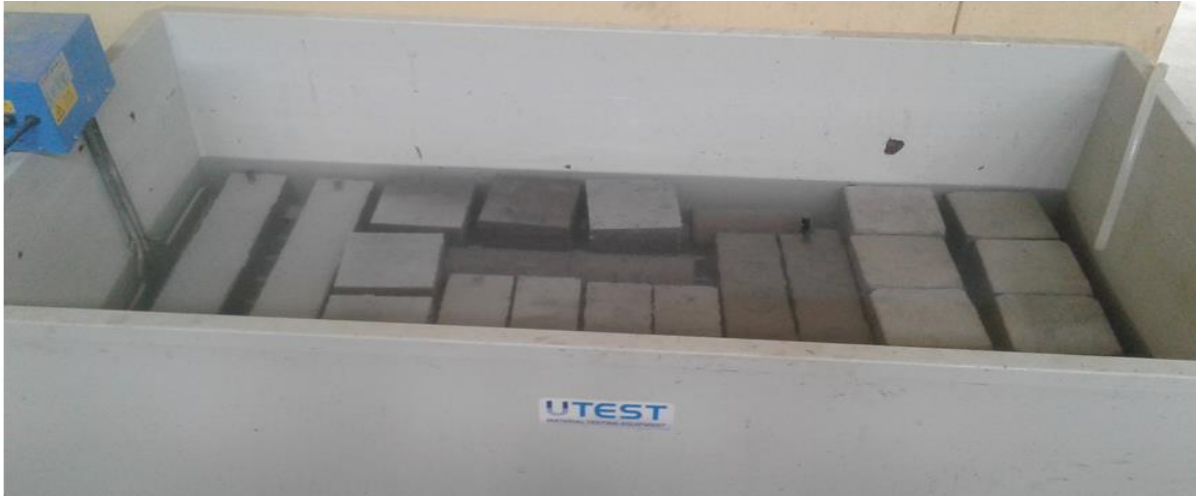
Figure 3. 12: Curing of beams, cubes and cylindrical specimens in the curing tank
