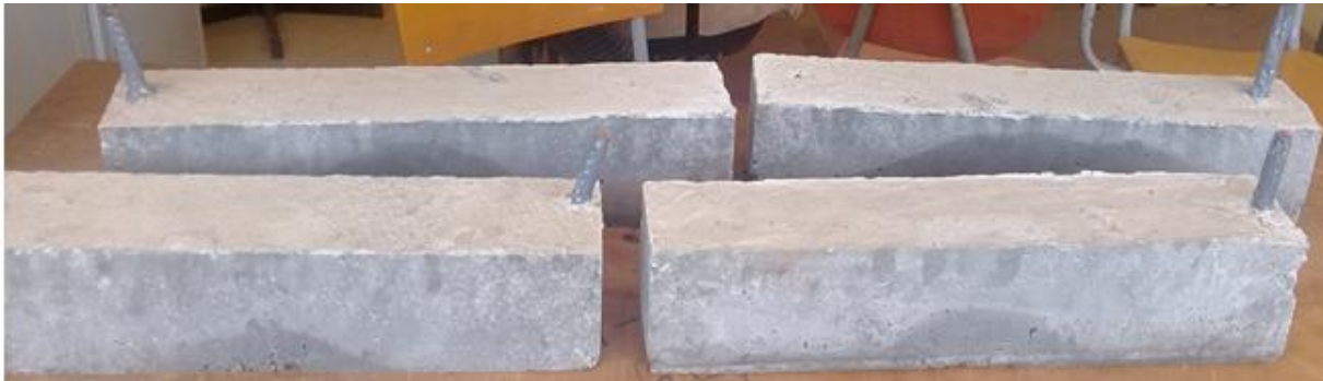
Figure 3. 13: RC beams after 28 days of curing
