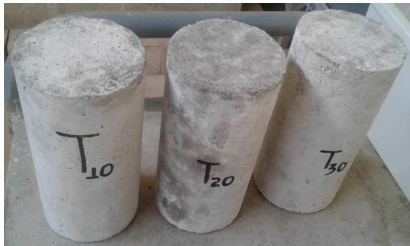
Figure 3. 19: Cylindrical specimens for splitting tensile strength test of plain concrete
