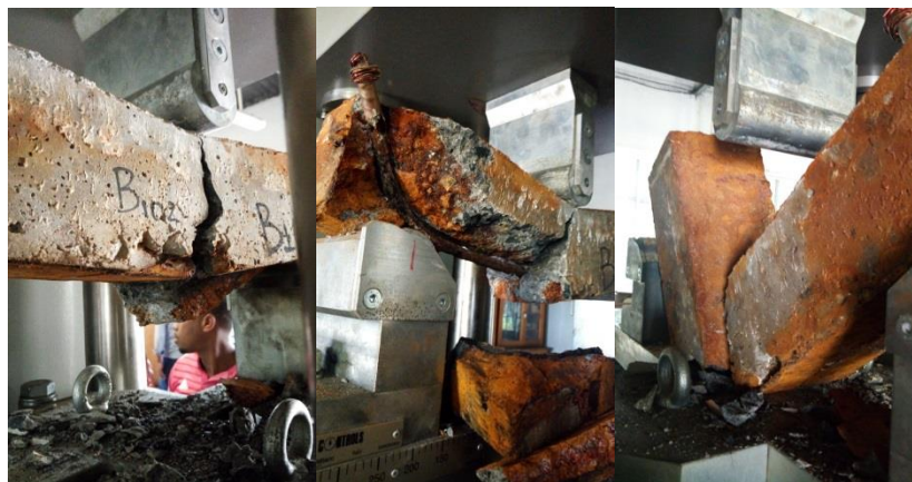
Figure 4. 22: Types of corroded beam failures (plain RC beam)
