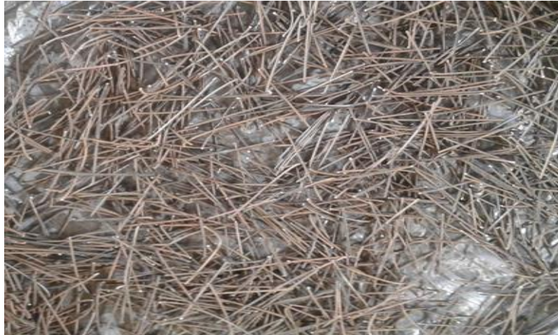
Figure 3. 7: Steel fiber extracted from used tire.
