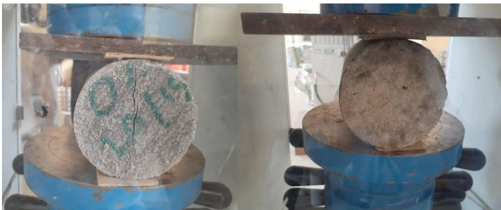
Figure 3. 21: Plain and SFRC cylindrical specimen in tensile splitting testing machine
