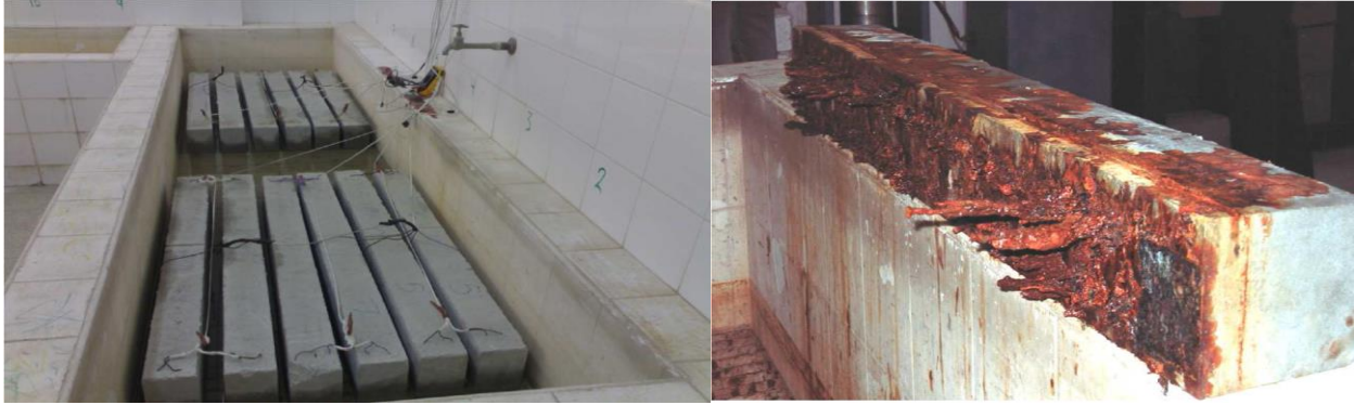
Figure 2. 9: Electrical Connection of and Rust on beams at the end of corrosion process (62)
