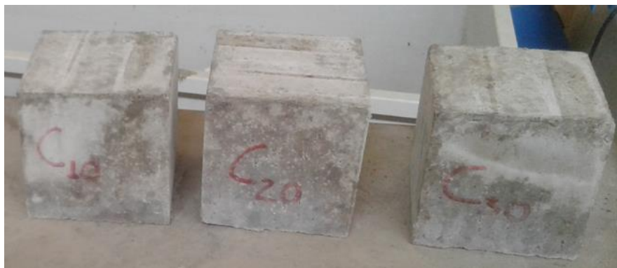
Figure 3. 14: Cubic specimens for compressive strength test of plain concrete
