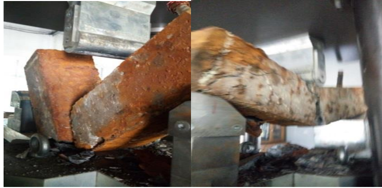
Figure 4. 14: a) Brittle failure b) Ductile failure
