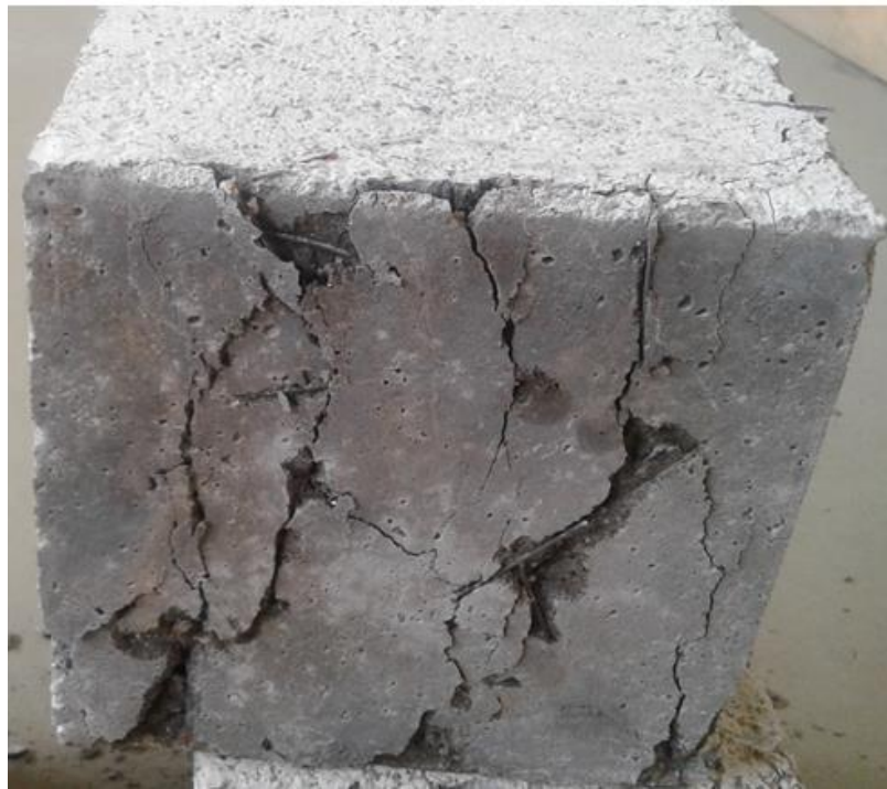
Figure 4. 3: Steel fiber reinforced concrete crushed cubic specimen
