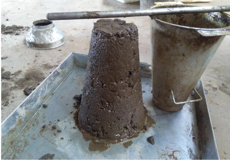
Figure 3. 11: Plain concrete slump (true slump)
