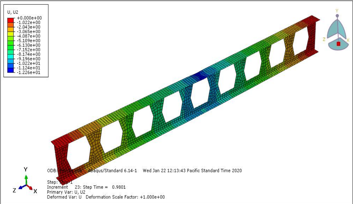
Figure D-6 Analysis of hexagon opening
