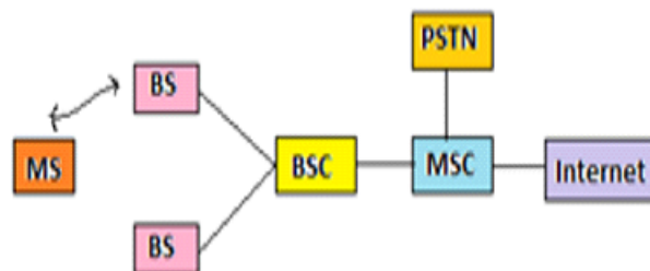
FIGURE 2.1: Architecture of Advance Mobile Phone System [19]
