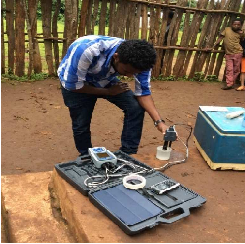
Onsite measurement of non-conservative parameters
