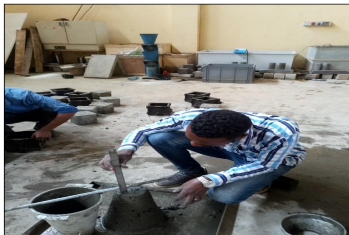
Figure 4.2: Slump Value Test
