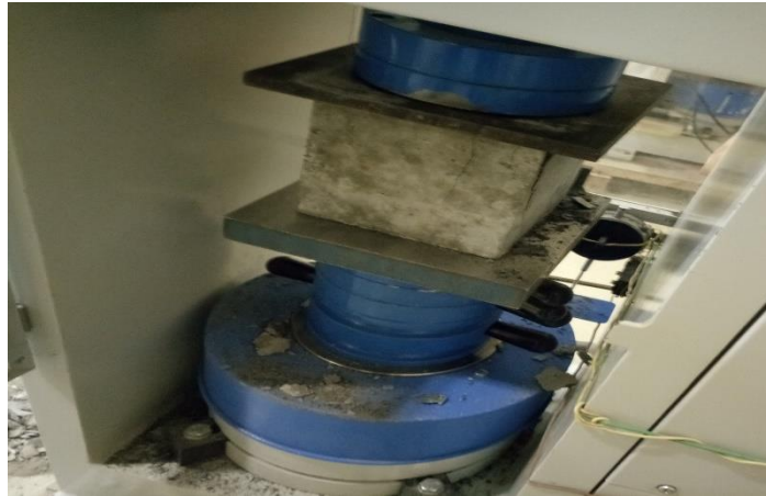
Figure 4.8: Compressive Strength Test
