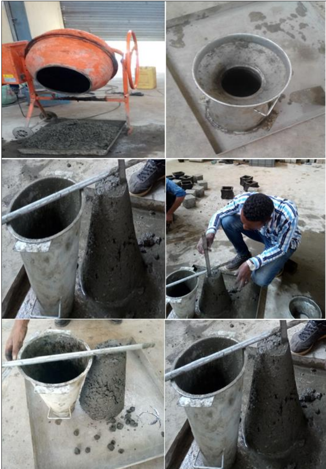
Workability of Fresh Concrete Test
