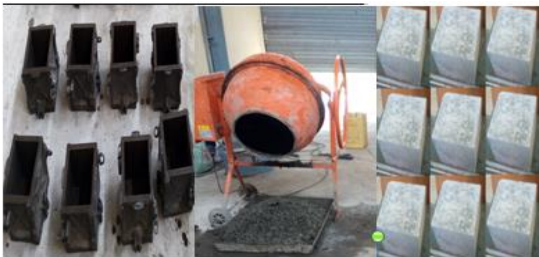
Figure 3.7: Concrete mixing and Casting processes
