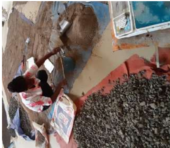
Figure 3.3: The compacted and loose unit weight of fine aggregate
