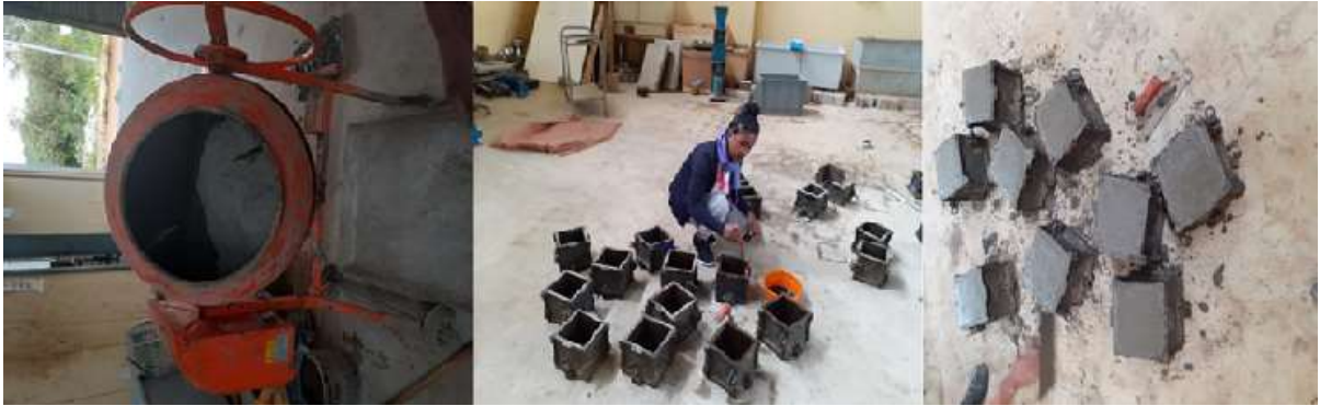
Figure 3.5: Mixing of ingredients, Oiling of mold and casting of specimen
