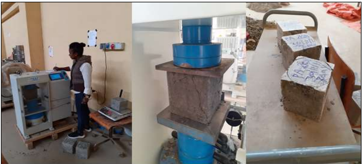
Figure 4.9: Compressive strength of concrete being test
