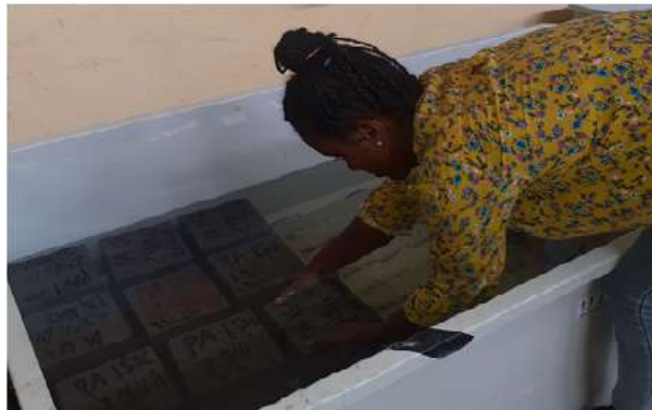
Figure 3.7: Curing of concrete cubes
