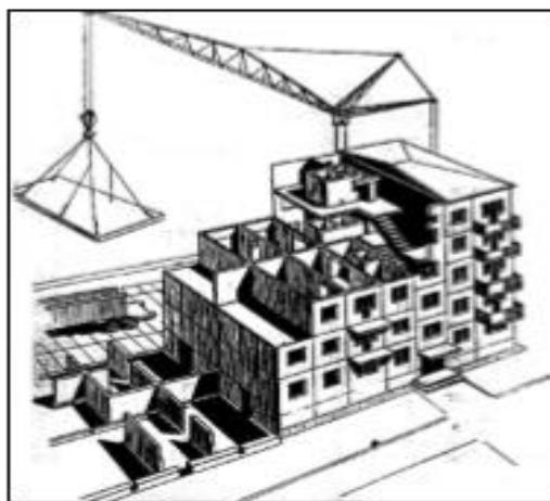
Figure 2.1 large-panel concrete building under construction
