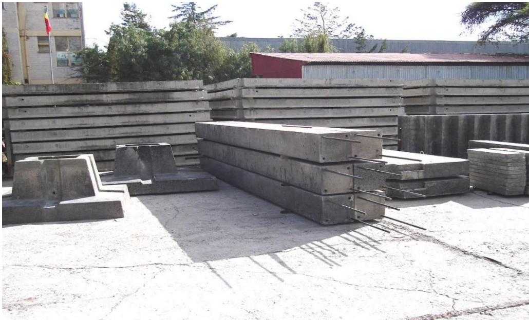
Figure 4.7: Precast concrete building elements
