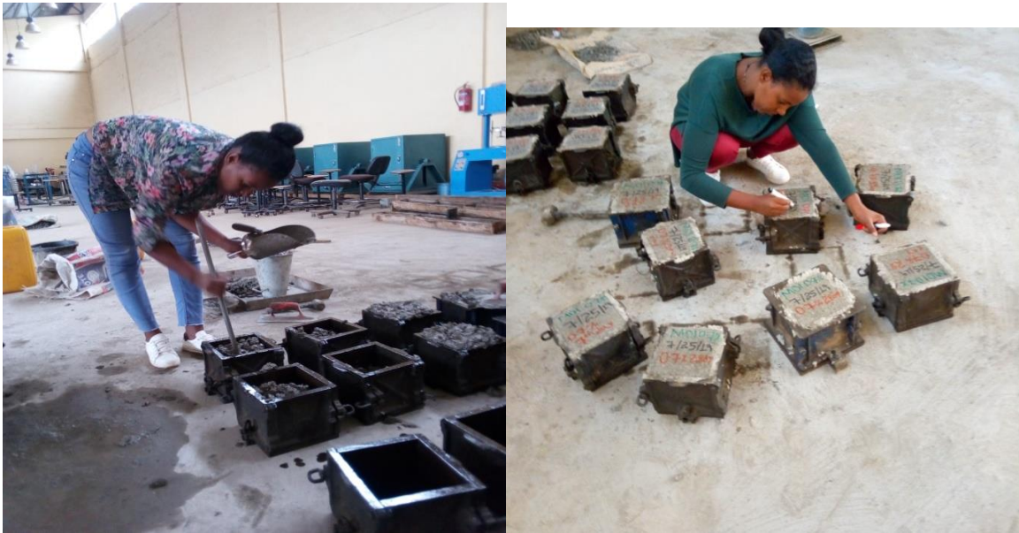
Figure 3.12 Concrete Casting Processing
