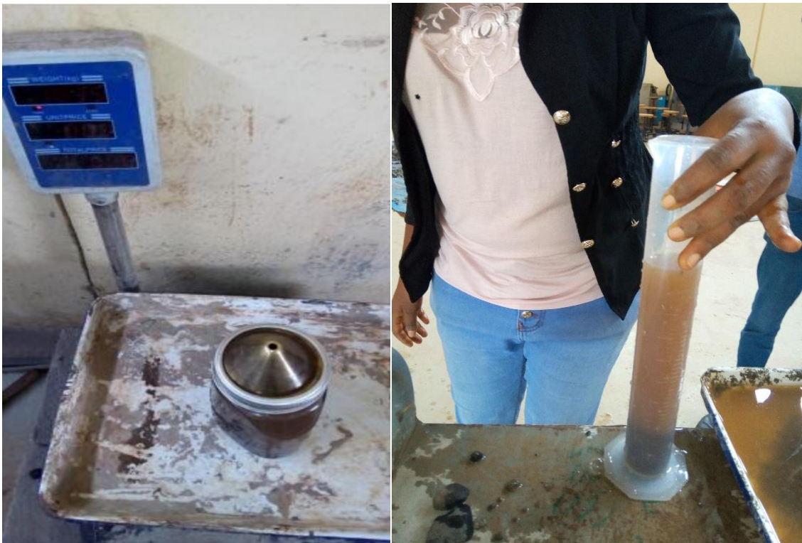
Figure 6 specific gravity test and silt content test of fine aggregate
