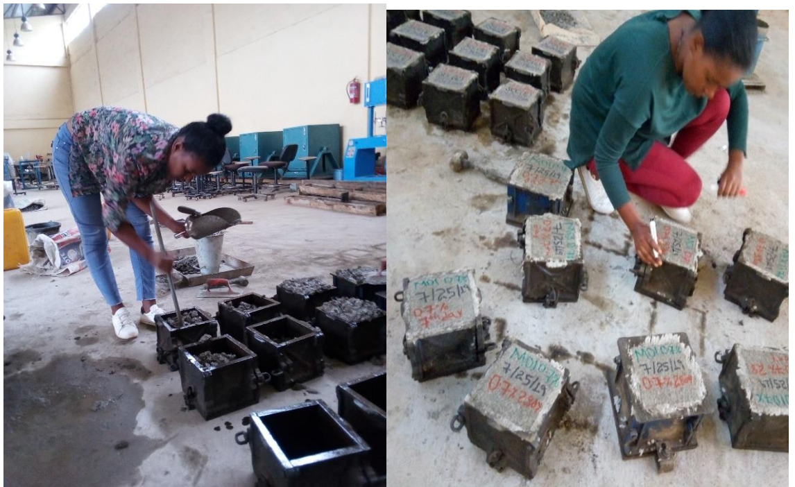
Figure 14 Casting of Concrete
