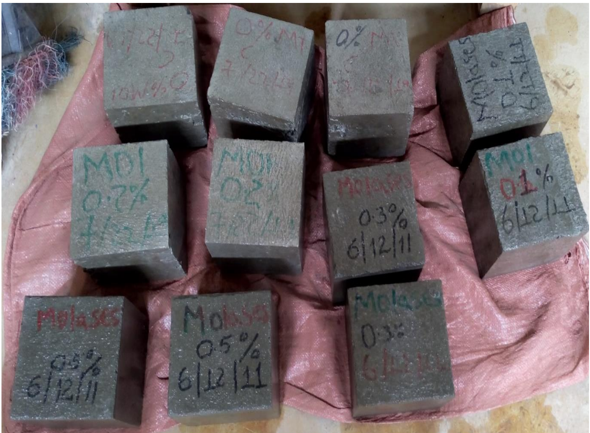
Figure 16 Surface drying of concrete mold
