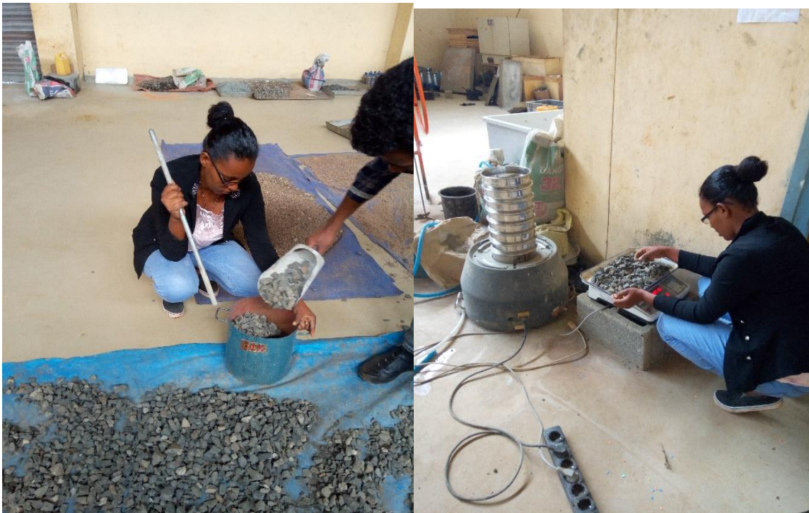
Figure 7 washing of coarse aggregate to make free of clay lump
