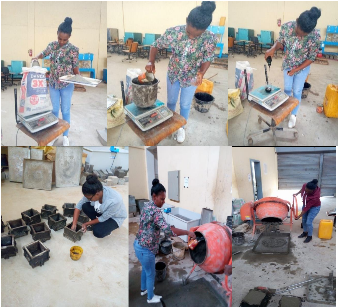
Figure 3.10 Concrete Mixing Process
