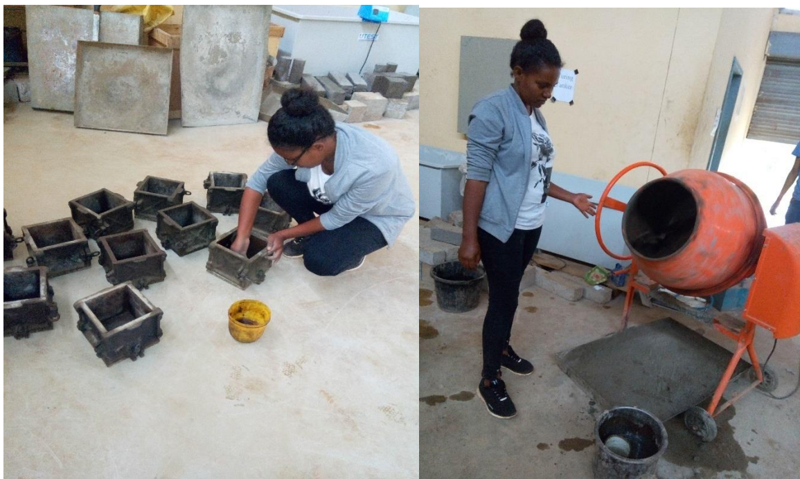
Figure 10 coating molds with oil and cleaning concrete mixer
