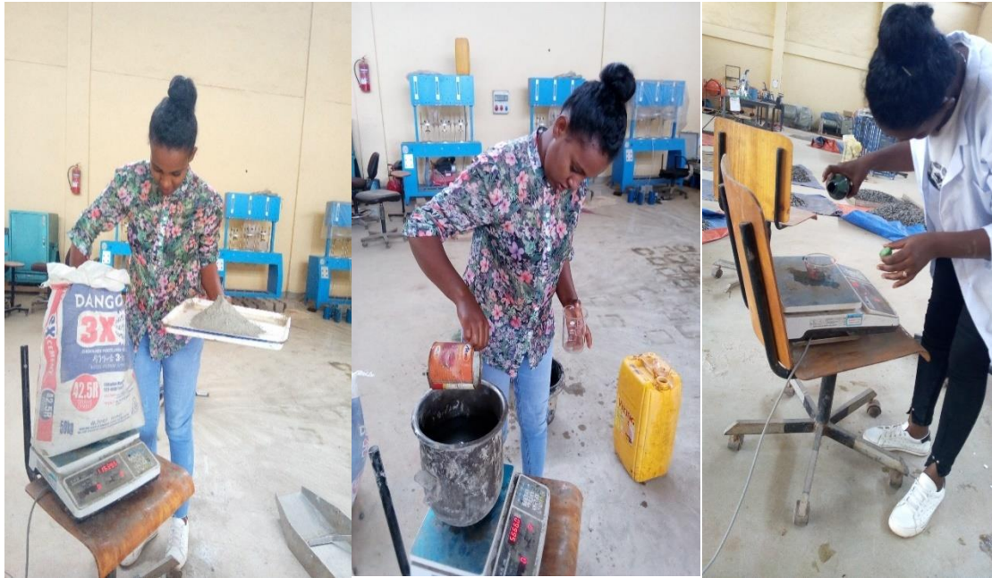
Figure 11 measuring concrete ingredient
