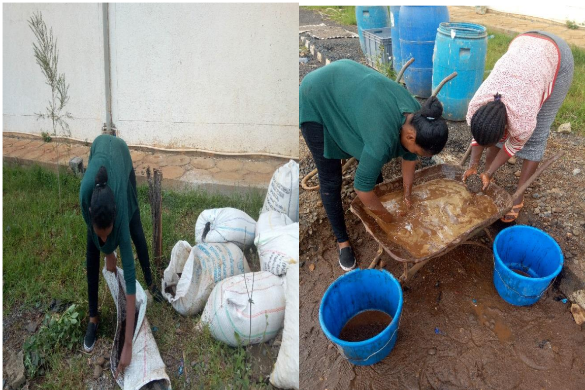
Figure 4 washing of sand to make free of silt and clay
