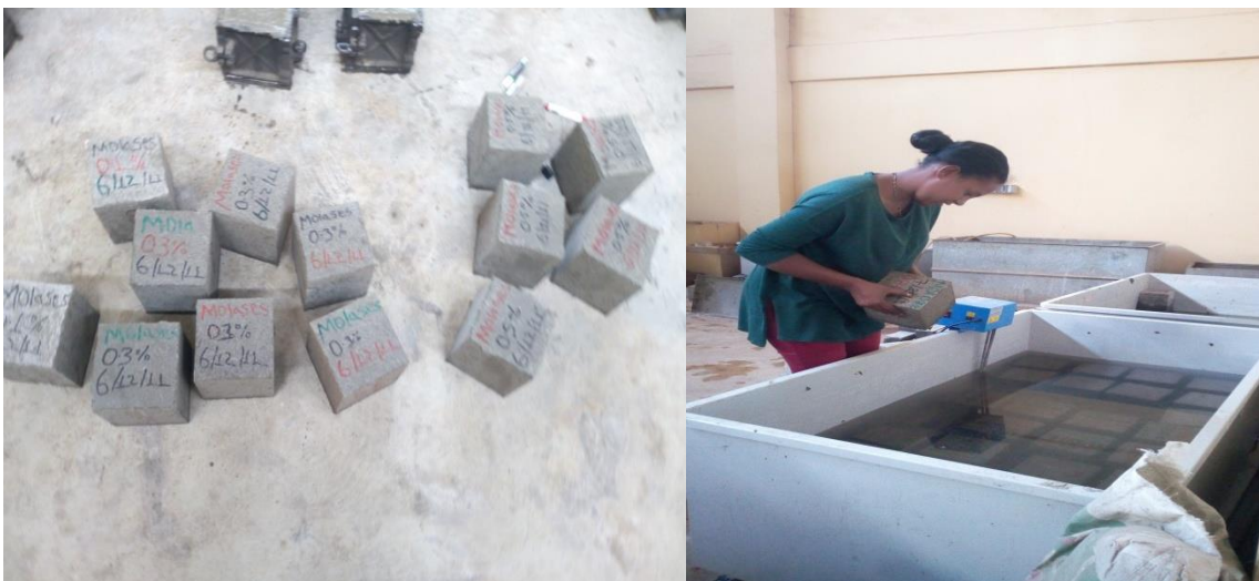
Figure 3.13 Removing of Concrete Cube from the mold & Immersion into curing water tank
