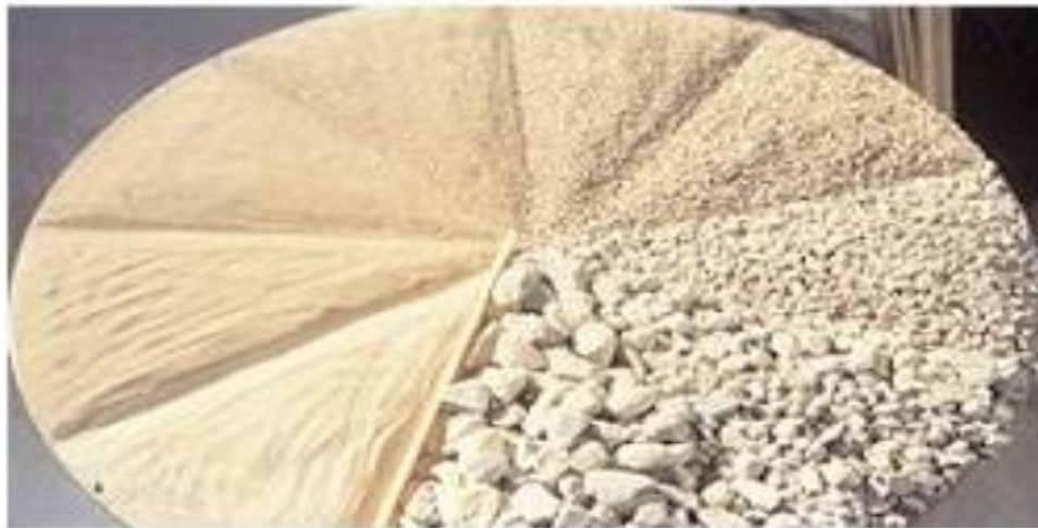
Figure 2.2 Range of particle sizes found in aggregate for use in concrete (Steven H. and Kosmatka B. K.). Fine aggregate is generally sand, but more precisely it is that material of which 95% passes through a No. 4 sieve. A No. 4 sieve consists of a wire mesh with wires spaced at 1/4 in. On center, because the wires have a
