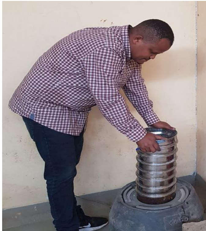
Figure E.1: Sieve analysis of aggregate samples used
