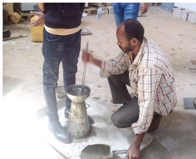
Figure 3.4: Filling the slump test cone with three layers and rodding each layers 25 times
