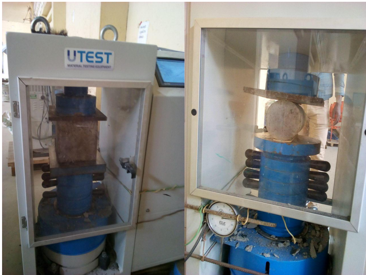
Figure E.5: Compressive strength and tensile strength test set up
