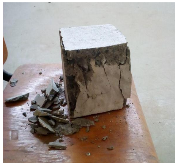
Figure E.6: Concrete specimen after testing
