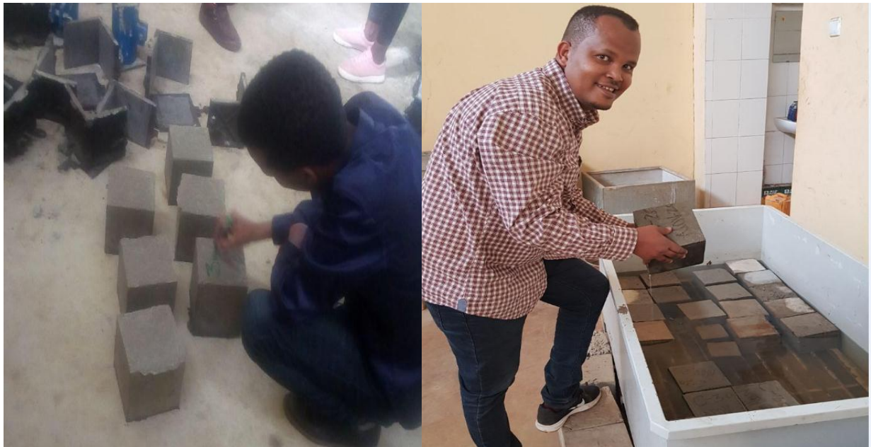
Figure 3.3: (a) Writing the identification code on the specimens (b) Curing in water tank
