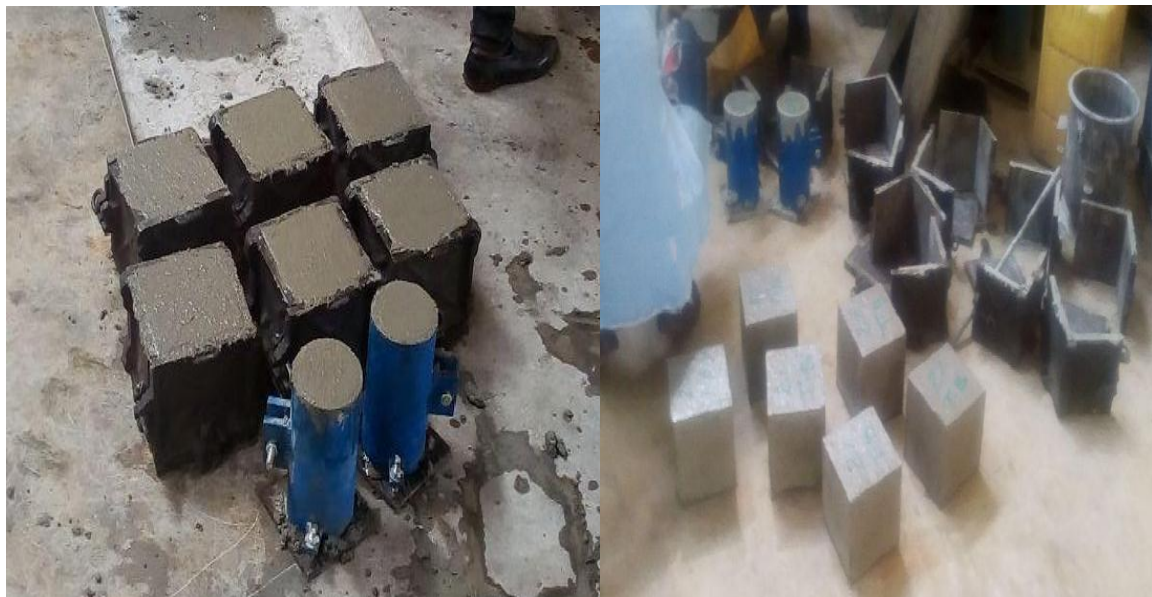
Figure E.2: Moulding and demoulding of concrete specimens
