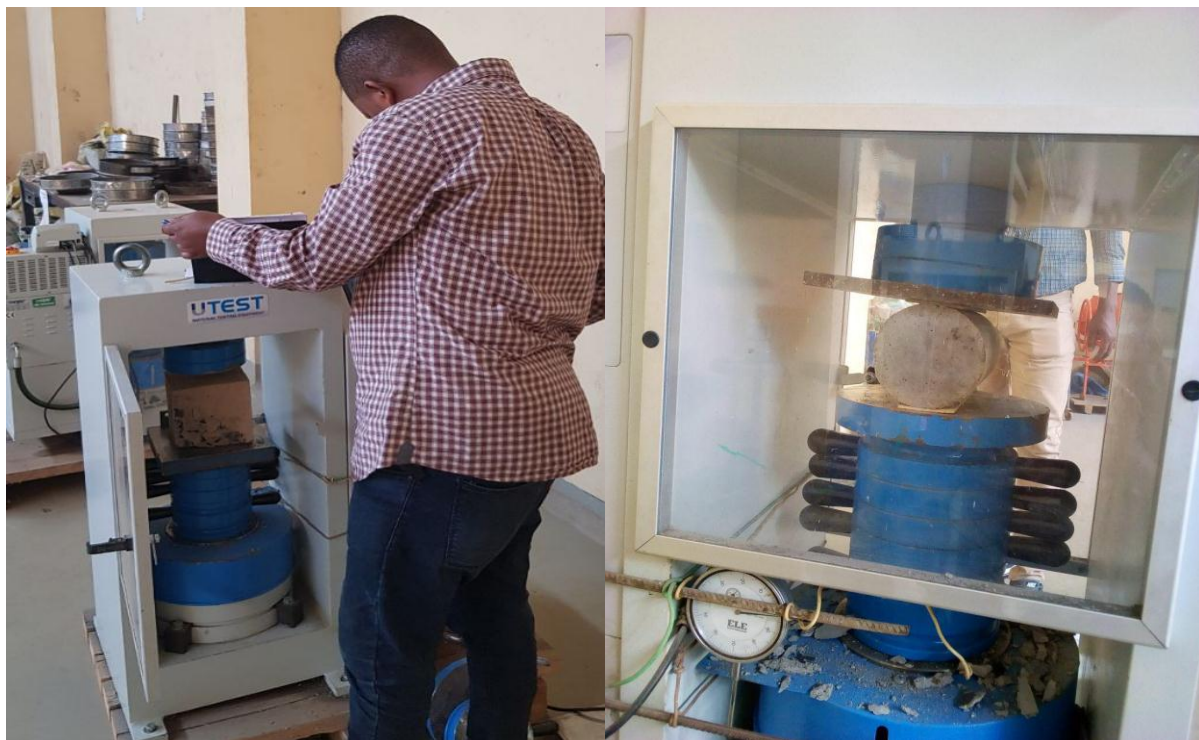
Figure 3.5: Compressive strength and split tensile strength test set up
