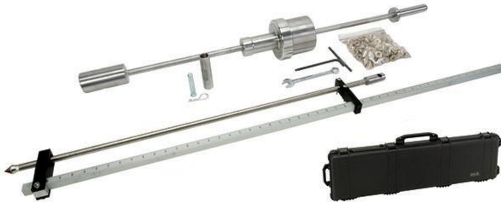
Figure 2. 1 DCP test equipment
