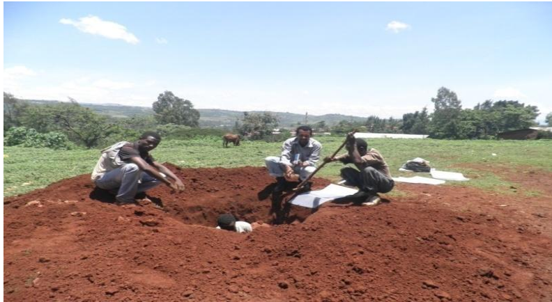
Fig 3.2 Test pit excavation at Agaro
