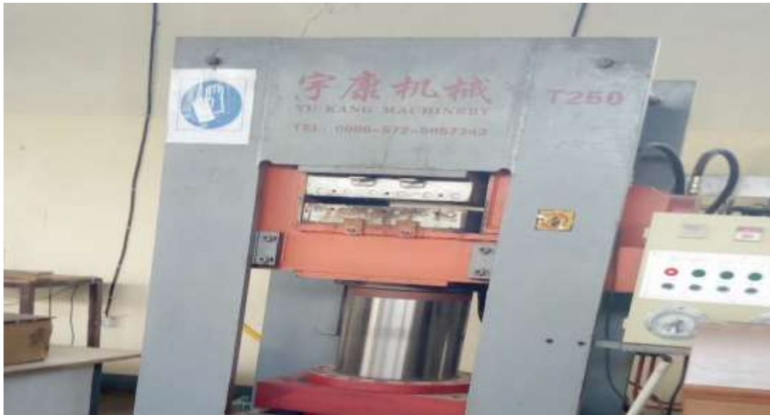
Figure 3.8. Standard Hydraulic Press for curing in African bamboo
