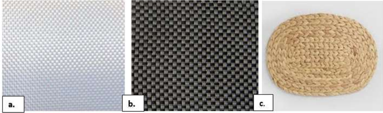
Figure 2.2.a). Glass fiber b). Carbon fiber c). Natural fiber [21]
