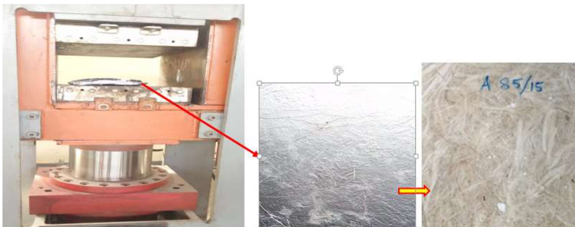
Figure 3.9. Releasing the cured sample from the mold plate and removing aluminum foil from sample
