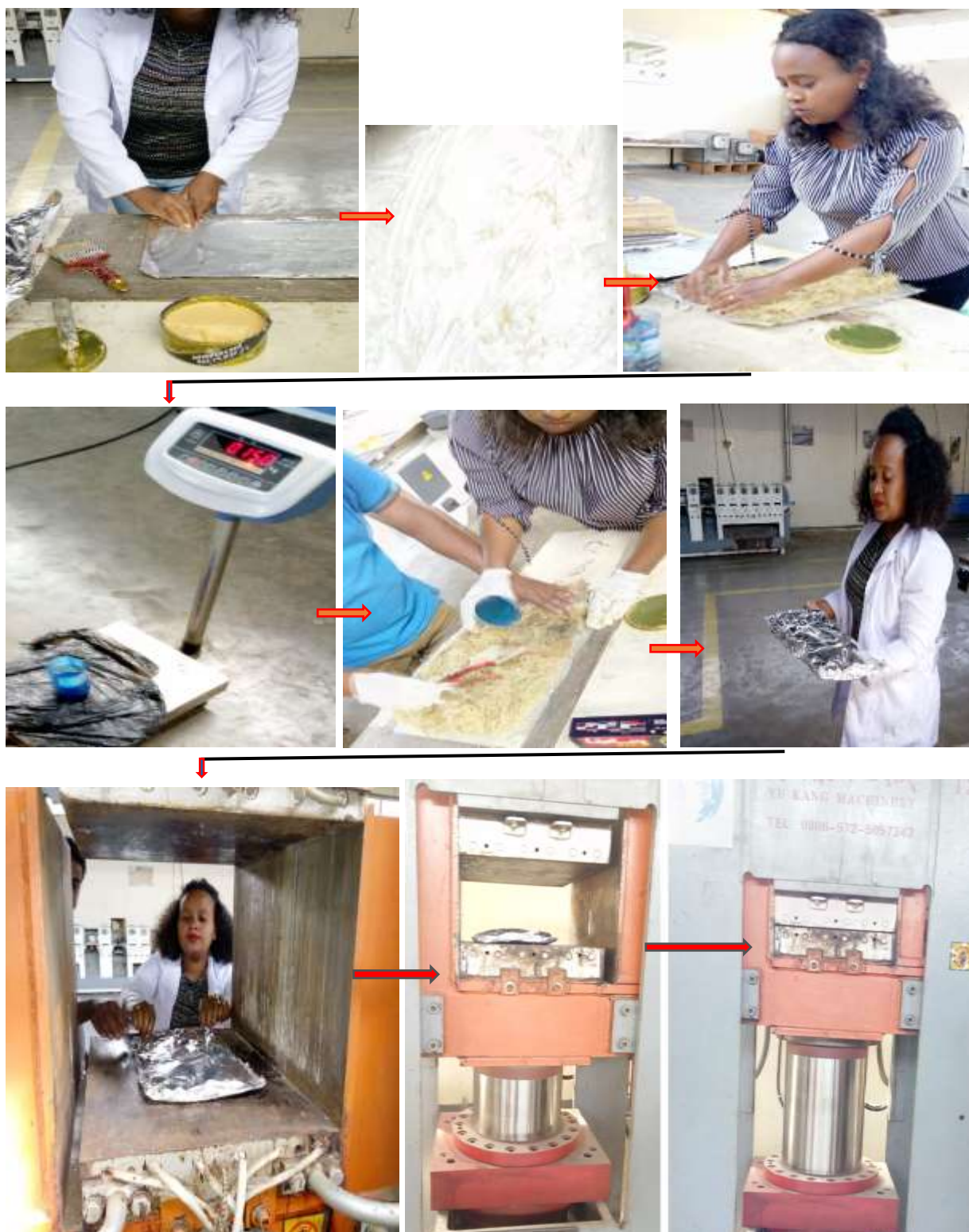
Figure 3.7 Palm and Pineapple fiber- epoxy resin mixture in the mold surface at African bamboo lab
