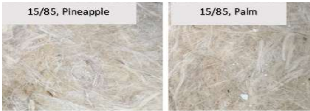
Figure 3.10. Prepared samples from pineapple and palm leafs
