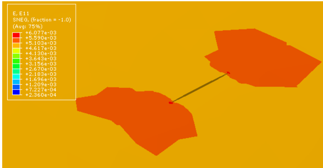
Figure 4. 26 Strain at the crack tip under thermal stress
