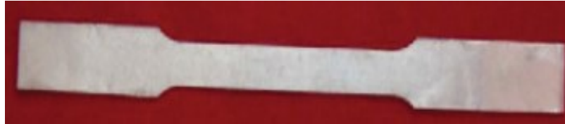
Figure 3.5 Specimen for the tensile test
