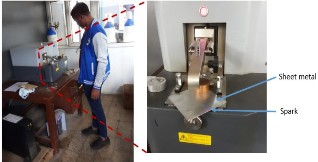
Figure 3.1 Spectromax x Ametek metal analyzer (Ethiopia commodity assessment enterprise)
