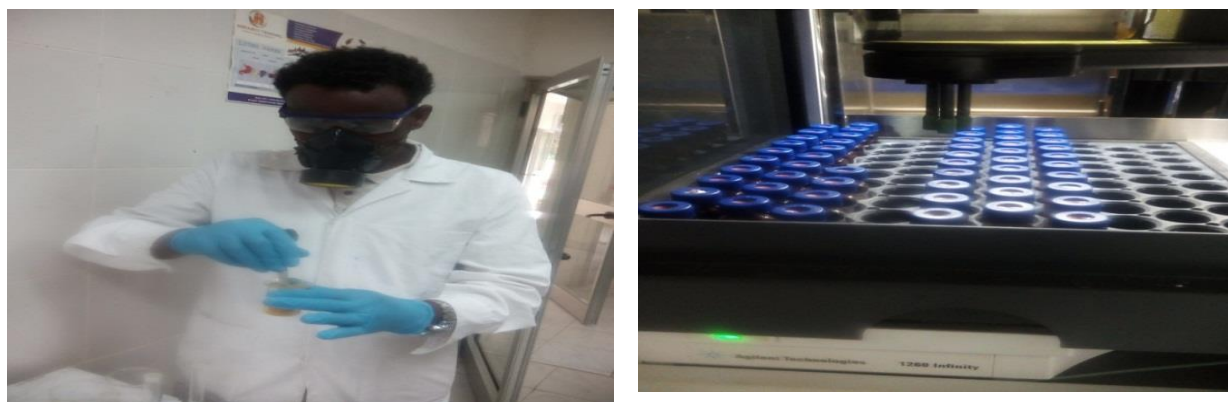
Figure 5. Honey sample processing in HPLC machine to calculate reducing sugar and sucrose
