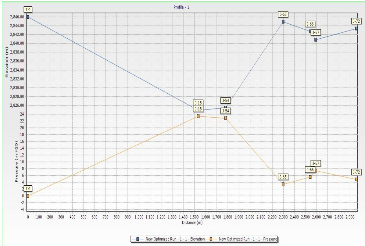
Figure 4. 4 Profiles of nodes showing distance from storage tank-1 (T-1)
