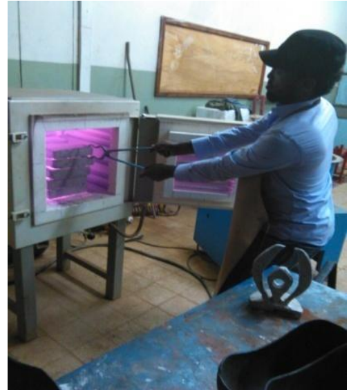
Photo-6 firing of clay bricks in furnace
