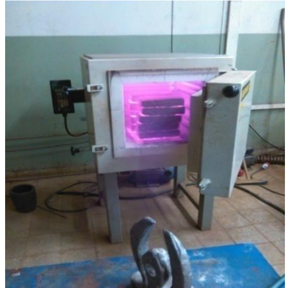
photo-10 high temperature furnace
