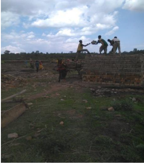
Photo-9 Traditional piling of brick for firing
