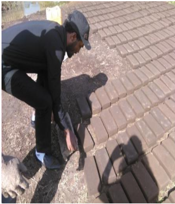
Photo-15 Air dried Bricks
