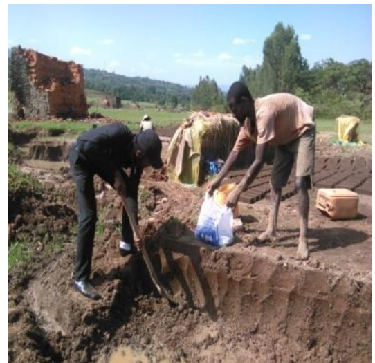
Photo-4 soil sampling for physical property test
