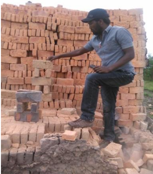
Photo-7 under burned brick kilns
