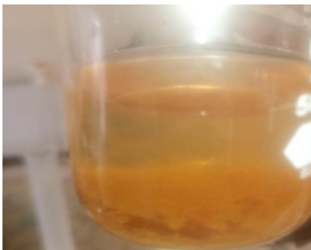
Figure 8: Light brown Precipitate of ferric benzoate
