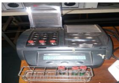
a) Thermostat digester
