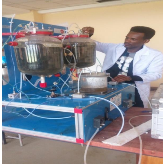
Figure 3.4 Anaerobic digester used in laboratory
