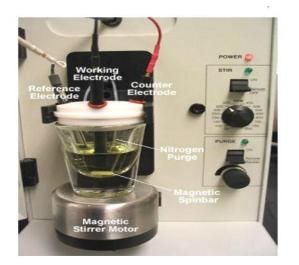
Figure 3: Typical electrochemical cell composed of three electrode systems for voltammetry
