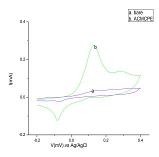
Figure 4. Cyclic voltammogram of a) 0.1mM AA (pH 4.5) UMCPE and b) 0.1mM AA (pH 4.5) ATMCPE, scan rate 100 mVs-1
