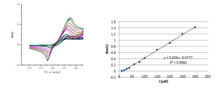
Figure 8. Cyclic voltammetry voltammograms for anthraquinone modified electrode containing different concentration of ascorbic acid scan rate 100mv/s
