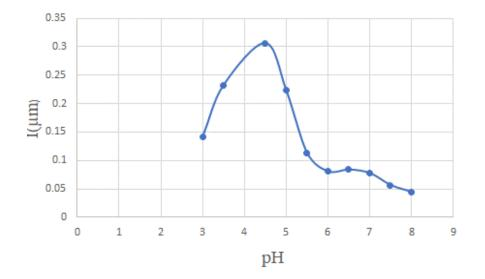
Figure 5. The relationship between the redox peak current of AA and buffer pH values
