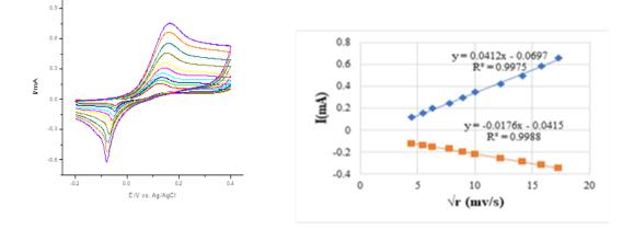
Figure 6. CV voltammograms of 0.1mM AA at ATMCPEs in PBS buffer at pH 4.5 at different scan rates, from 20-300 mVs-1 (Inset: The plot of Ipa and Ipc *vs.* v1/2)
