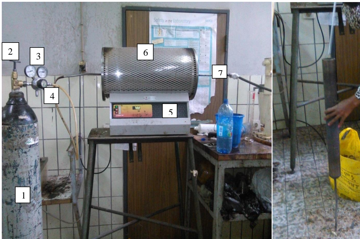
Figure 3: Tube Furnace: experimental set-up of Biochar production at 350°C, 450°C and 700°C temperature for 2hrs. (1 N 2 cylinder, 2 valve, 3 pressure meter; 4 flow meter, 5 furnace, 6 sample, 7 stainless steel tube and 8 trap)
