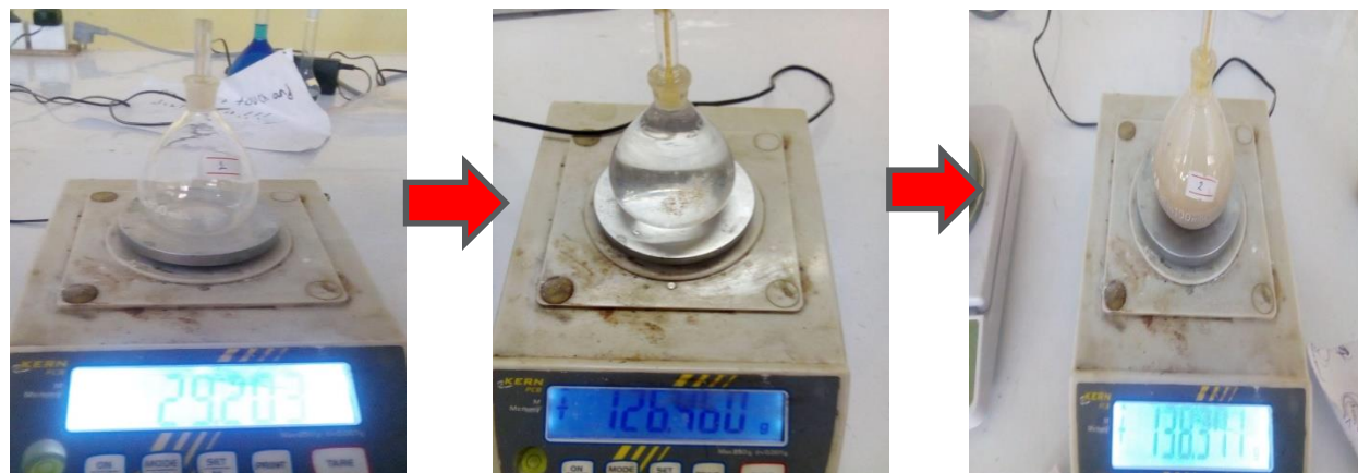
Figure A 3: Particle density for TMESP adsorbent using a pycnometer
