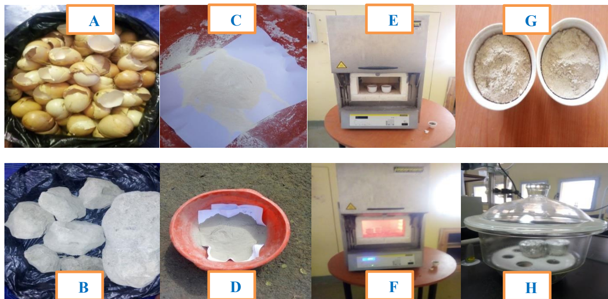
Figure 3.2: physical demonstration of adsorbent preparation: (A&B) Raw Materials of TM-ES, (C&D) powder of TM-ES, (E&F) calcination process, and (G&H) synthesized of TMESPs.
