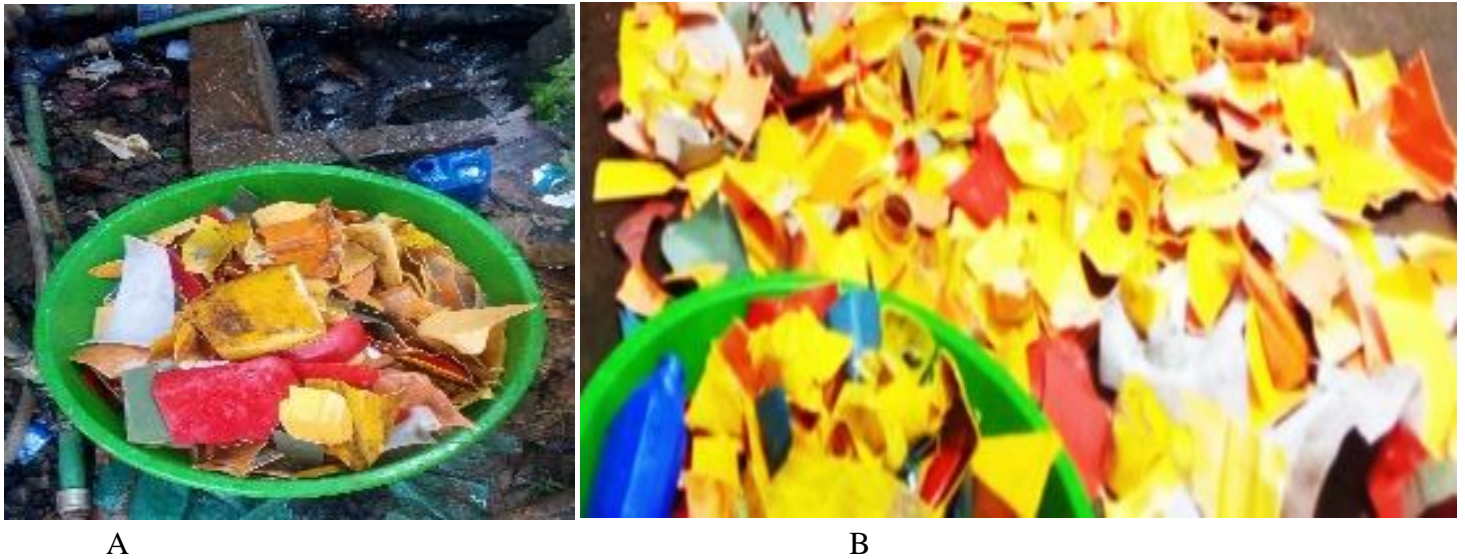
Figure 7. Washing A), and drying B) of HDPE waste plastics
