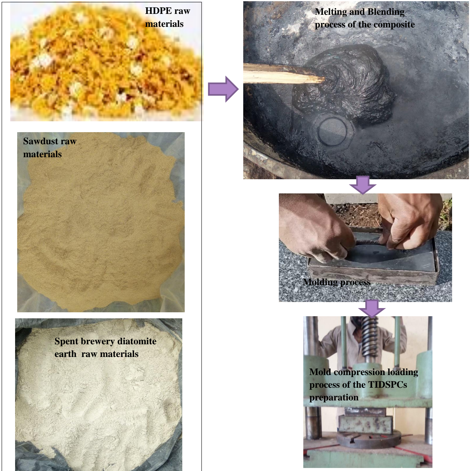
Figure B 6: Preparation of TIDSPCs thermal insulation composite materials
