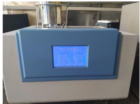
Figure B 1: Thermogravimetric (TGA) instruments used for thermal stability analysis in this study.
