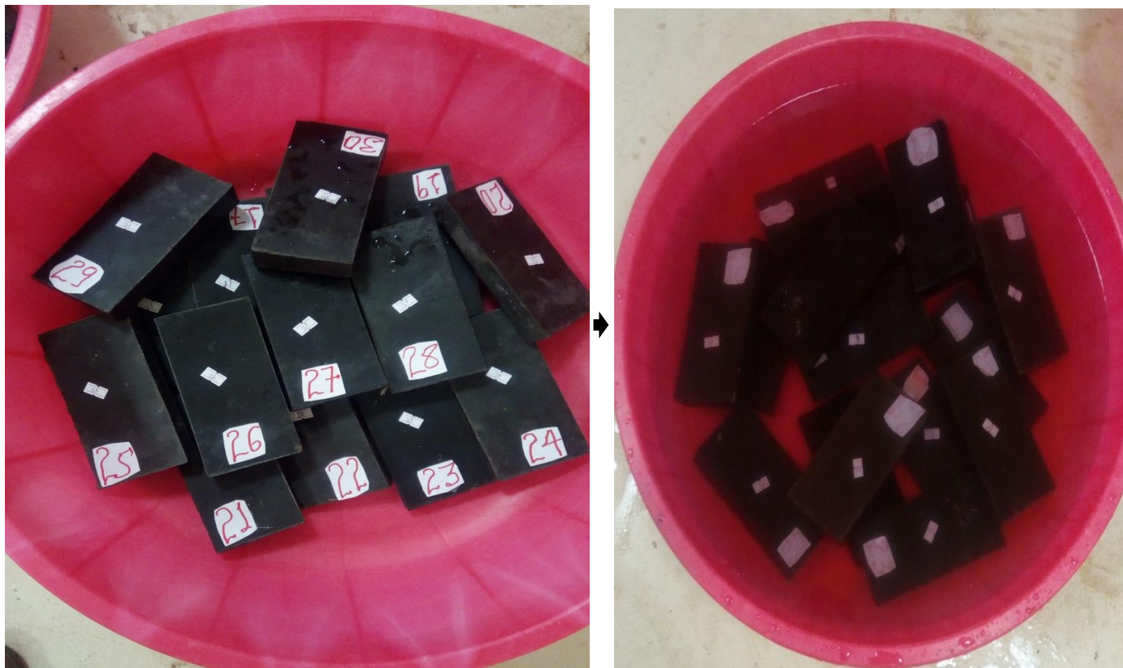
Figure 13. Water absorption properties test of TIDSPCs
