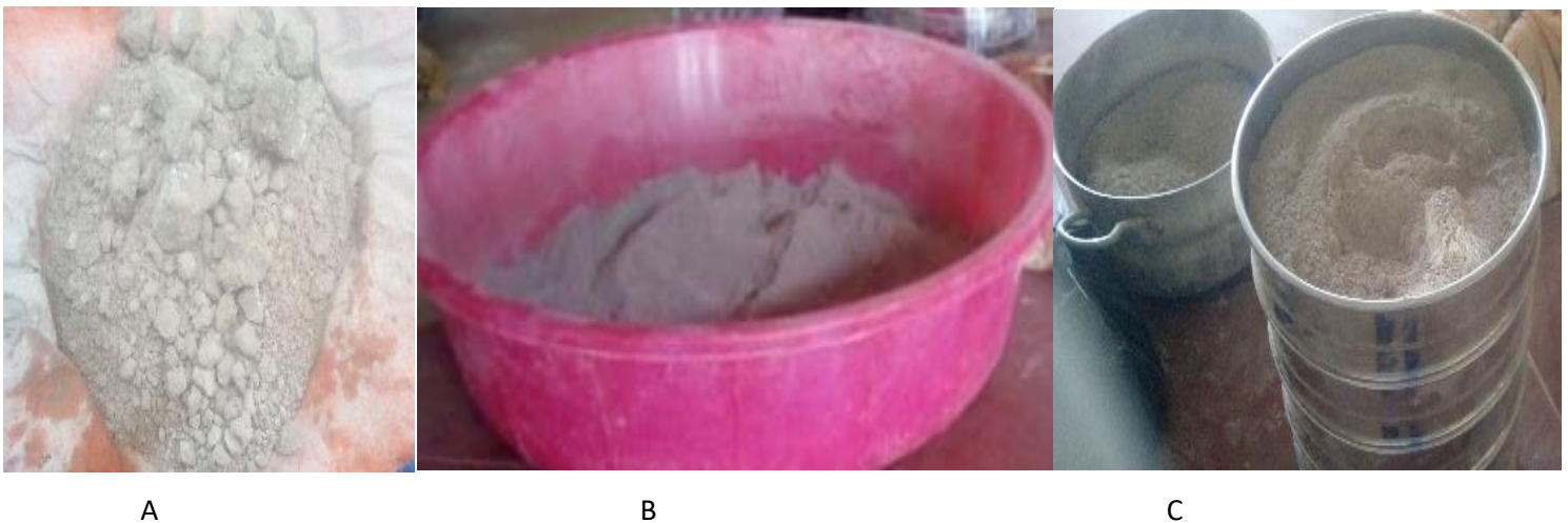
Figure 6. The raw A), the grounded B), and the sieving C) process of spent brewery diatomite earth material
