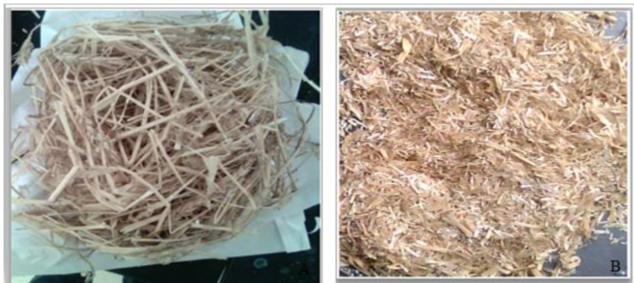
Figure 3.4: A. WS sample and B. washed and size reduced WS
