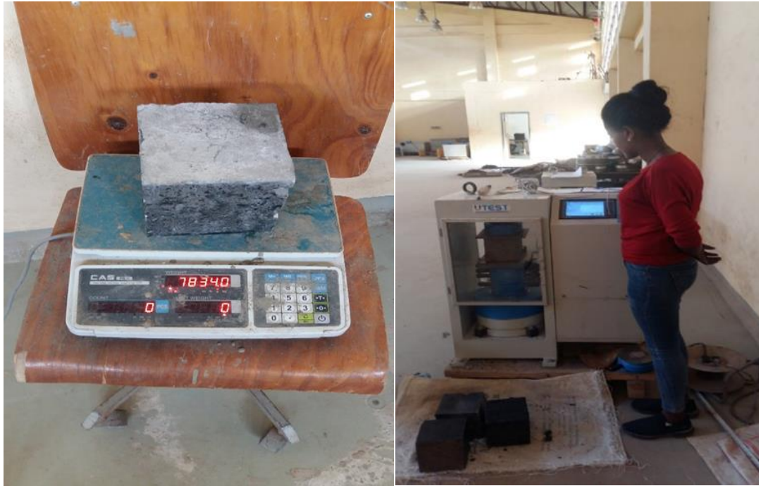
Figure 3. 6:Measuring of compressive strength
