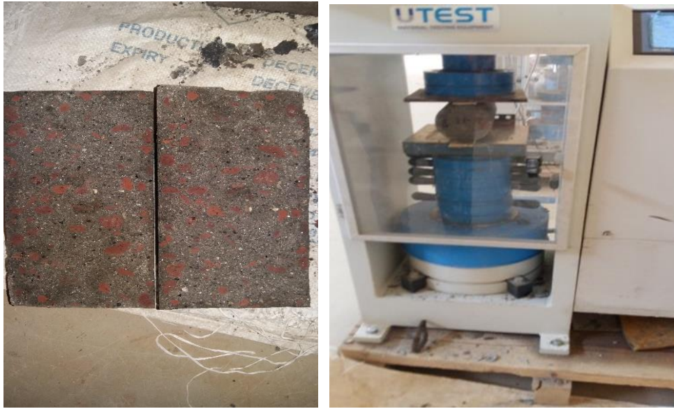
Figure 3. 7: Measuring split tensile strength
