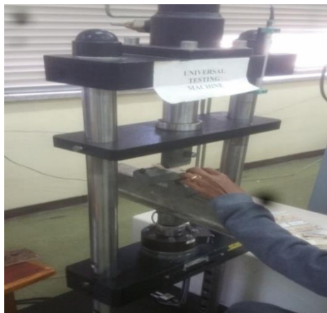
Figure 3.13 Typical specimens under flexural test
