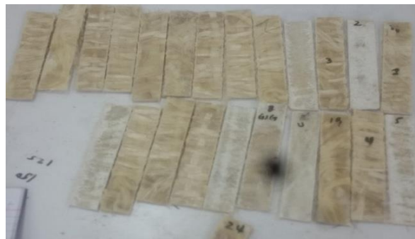
Figure 3.9 Prepared specimens for tensile test
