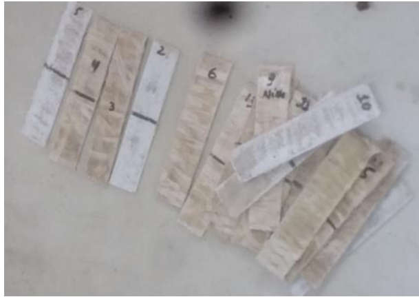
Figure 3.10 prepared specimen for flexural test
