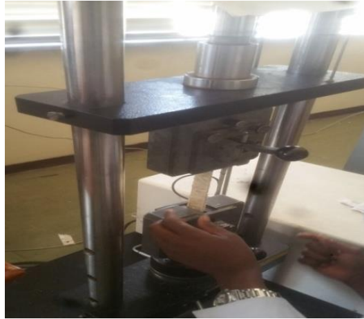
Figure 3.12 Typical specimens under tensile test
