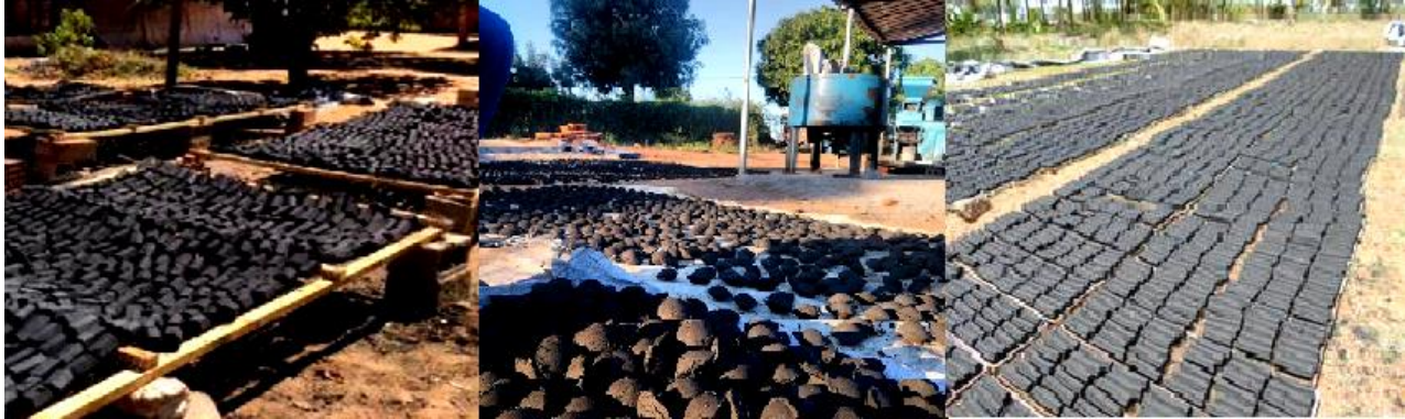
Figure 2.2: Drying briquette under the sun in Mozambique [26]
