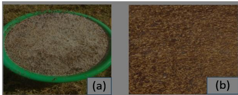
Figure 3.4: a) Coffee husk treatment with NaOH solution and (b) dried coffee.
