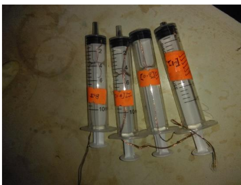
Figure 23: Chemically synthesized polyaniline as a working electrode
