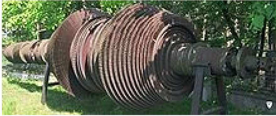
Figure 2.4: Parsons turbine from the Polish destroyer ORP Wincher
