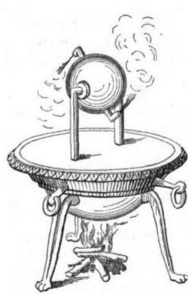
Figure 2.2: Herons idea for a steam turbine
